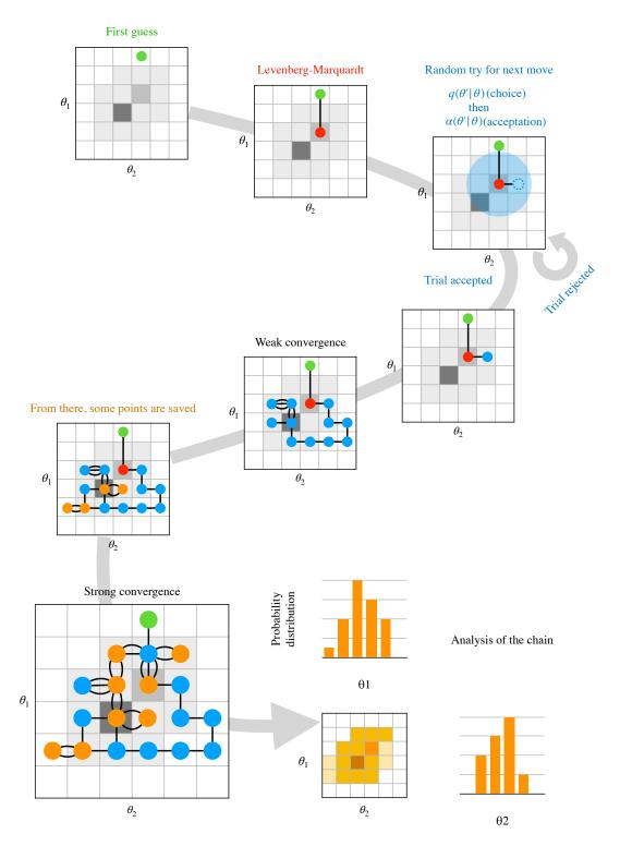
Figure 2.1 – Schematic of the procedure to retrieve the probability distribution of the parameters  $\theta_1$  and  $\theta_2$ . The maps represent the 2D histogram of the  $\chi^2$ . The Gibbs sampler prevents diagonal moves. The discretization is for better readability and is not a feature of the code.
