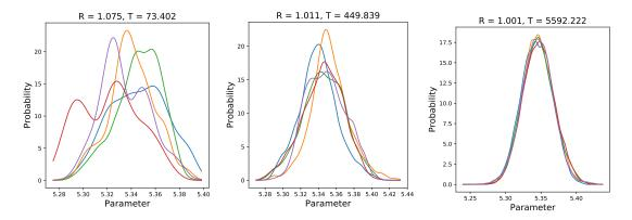
Figure 2.2 – Example of the probability distributions function of 5 chains that respectively have not converged, have weakly converged and strongly converged, according to the Gelman-Rubin statistics.
