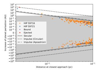
Fig. 8. Periastron increase with respect to the distance at closest approach, from N-body simulations (dots) and theoretical approaches (lines), for the closer fly-bys, and for an initial planetary apoastron of 1,000 au. The grey part corresponds to a periastron change inferior to +1 au, which will not secure the planet stability.
