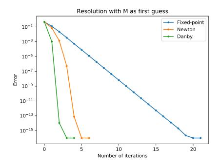
Figure 31 – Three methods to solve Kepler equation, with initial guess u = M, and for medium eccentricity e = 0.5. A more complex initial guess can reduce the number of steps by 1 or 2.
