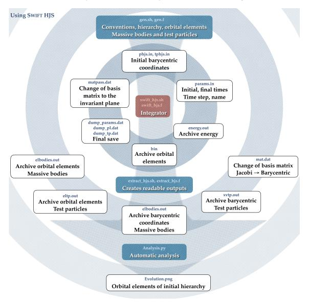
Figure 1.7 – Schematic of the inputs and outputs of SWIFT HJS. The user inputs are filled in gen.sh and params.in.
