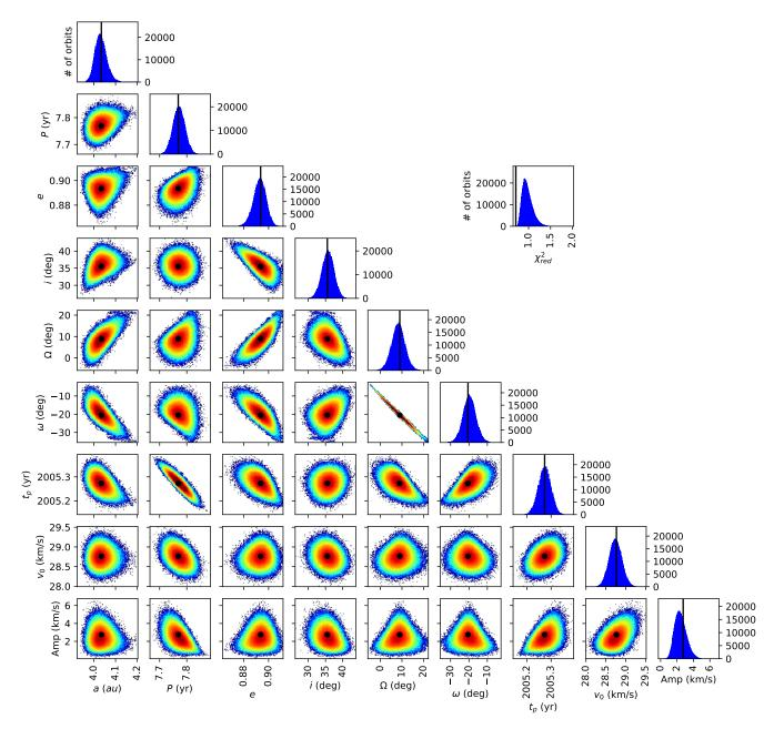
Fig. B.2. Distribution and correlations of each of the orbital elements fitted by the MCMC algorithm for system GJ 2060. The black lines and points depict the best fitting orbit (lower  $\chi^2$ ) obtained with the LSLM algorithm. The color scale is logarithmic; blue corresponds to 1 orbit and red to 1000.
