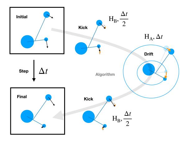
Figure 1.3 – Schematic of the kick-drift-kick procedure in the MVS framework.
