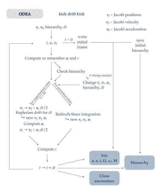
Figure 1.17 – Schematic of the core algorithm of ODEA.
