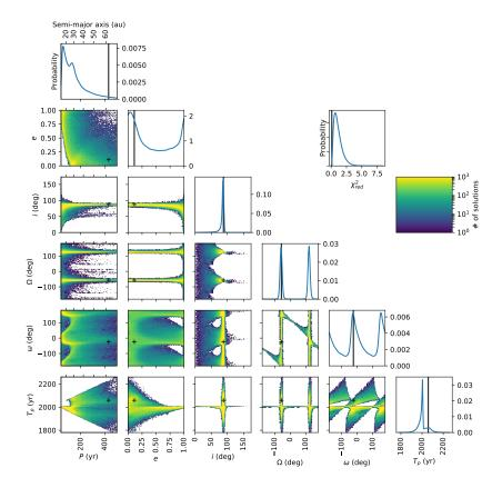
Figure 2.14 – Corner plot presenting the results of the MCMC orbital fitting procedure of HR 2562 A-b relative orbit. The black lines and crosses correspond to the results of the LM procedure (best fit).
