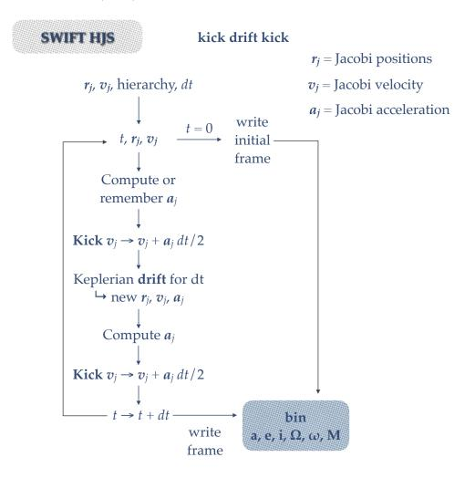
Figure 1.6 – Schematic of the core algorithm of SWIFT HJS.
