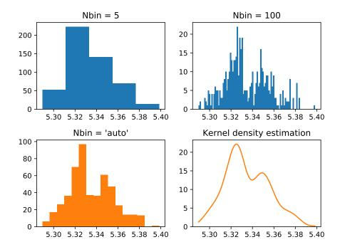
Figure 2.11 – Example of the importance of choosing an appropriate representation for the analysis of a probability distribution.
