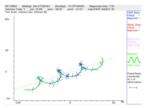
Figure 2.26 – HD 106906 apparent motion on the skyplane (around 3 years), fitted from the intermediate data from Hipparcos. The orbital motion induced by the planet is negligible over 3 years, so that the trajectory only corresponds to a linear proper motion with a parallactic component. The fit gives the parallax of the system and its proper motion with a precision of around 1 mas and 0.5 mas/yr respectively.
