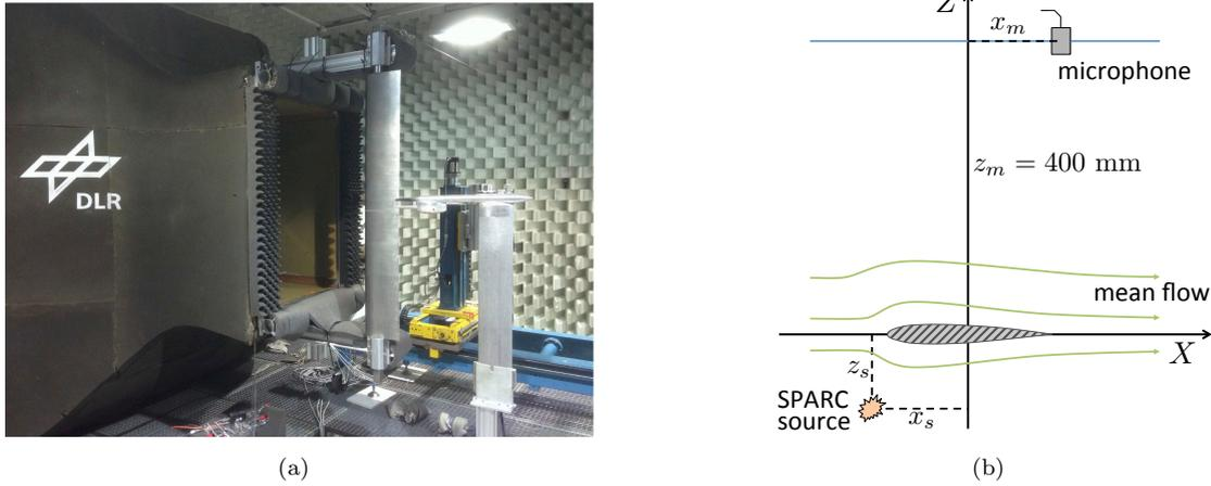
FIGURE 4.12: (a): Diffraction by a NACA0012 profile in the AWB wind tunnel. (b): Schematic view.
