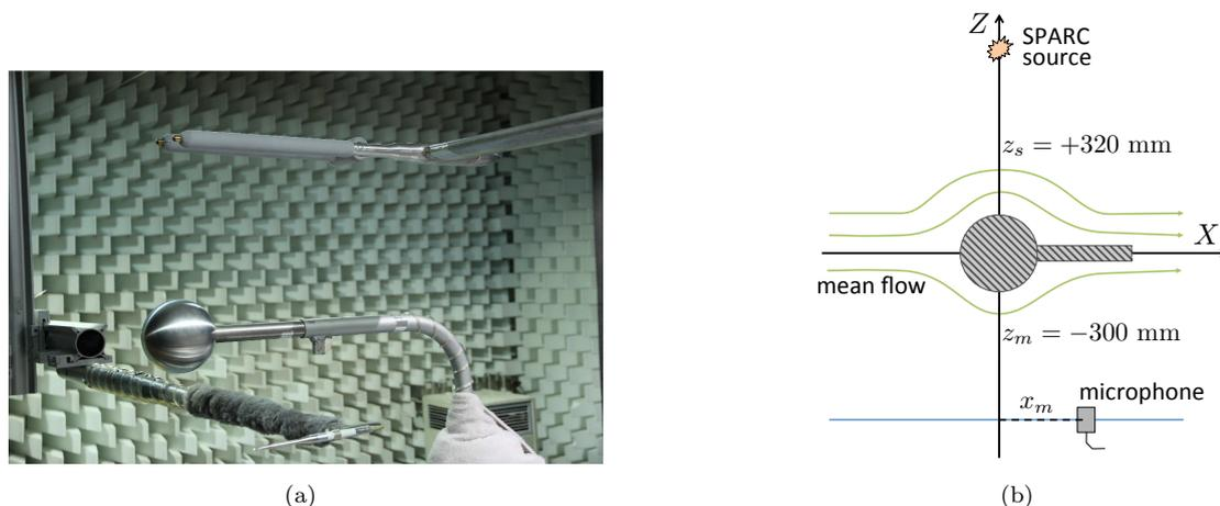
FIGURE 4.1: (a): Diffraction by a rigid sphere in the AWB wind tunnel. (b): Schematic view.
