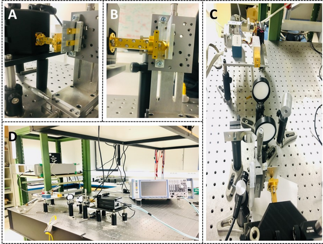
Figure 5.11 – Home-built optical set-up of the InAs membranes located at the T Hgroup. (A) InAs membrane positions. (B) Head of a heterodyne detection - Receiver system. (C) Caption of the entire optical THz and IR beam path. (D) Entire optic set-up with the synthesizer and the electrical spectrum analyzer.
