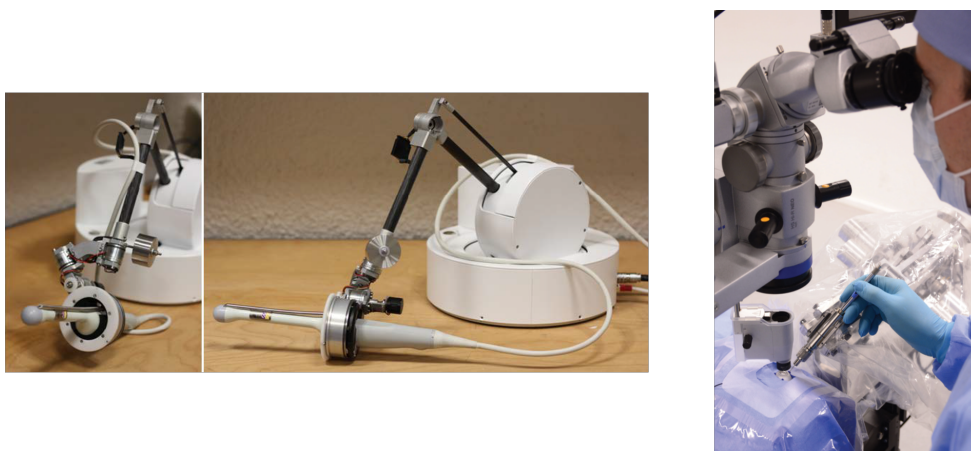
Figure 2.6 – Two parallel comanipulators with full-DoF control by the user: (left) Apollo [Poquet, 2014] (right) Gijbels et al. [Gijbels et al., 2018][Mynutia, 2017]
