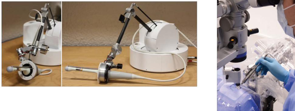
Figure 2.6 – Two parallel comanipulators with full-DoF control by the user: (left) Apollo [Poquet, 2014] (right) Gijbels et al. [Gijbels et al., 2018][Mynutia, 2017]
