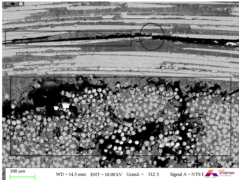
Figure 14: Two visible damages identified in sample d9v1 . Fibre-matrix de-cohesion can be seen in the square areas for both fibre orientations. Fibre failure can be seen in the circle area.
