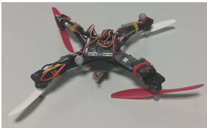
Figure 6.4 – Mosca quadrotor developed at GIPSA-LAB.
