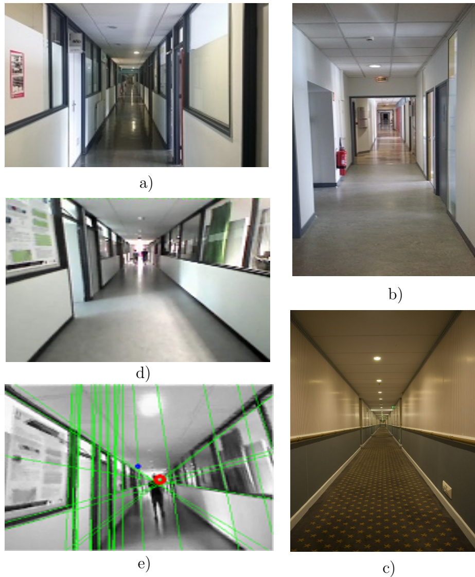
Figure 1.1 – Images showing a common corridor, it can be seen that lines can describe structure, doors, and windows. Figures a), b), and c) were taken with a smart-phone camera. Figure d) and e) were taken using a camera FPV with a 240x320 pixels. In c) some lines describing the structure are shown.
