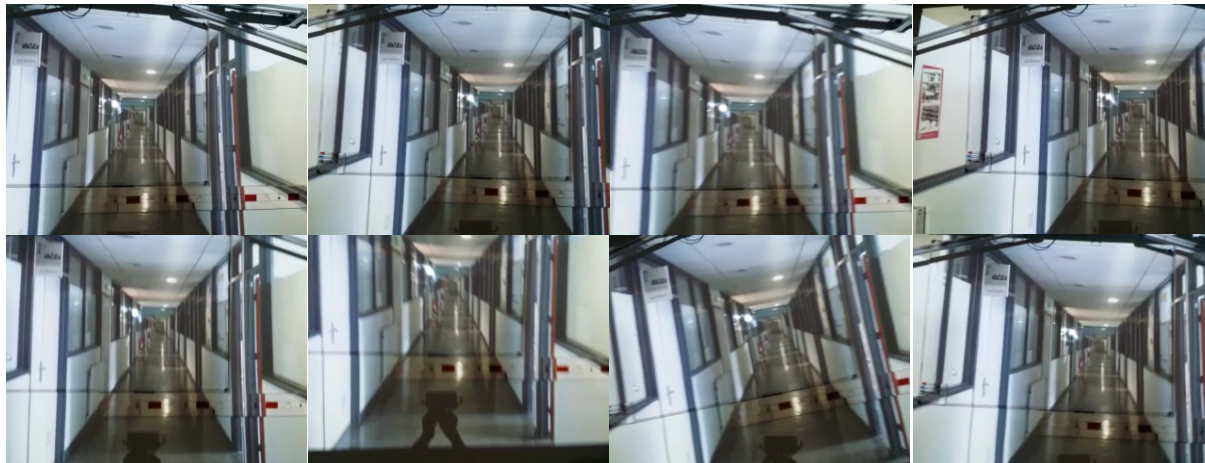
Figure 4.19 – A image, which was taken by a smartphone, was projected on wall using a commercial projector, then a video was taken by a smartphone whose some movements were made on yaw \psi , pitch \theta and roll \phi angles.
