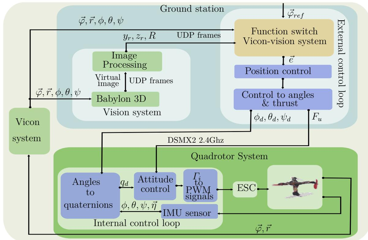
Figure 6.13 – General scheme of the vision system switching with the Vicon system using images from virtual world.
