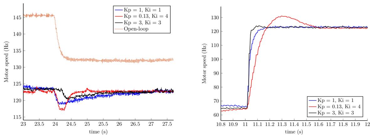
(a) Disturbance rejection. A 1 Volt drop is applied to the power supply, please note that the drop is not applied at the same time between the different experiments.
