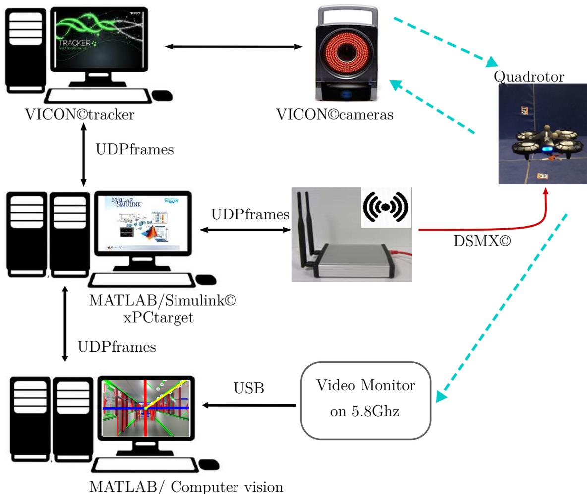
Figure 6.3 – Quadrotor control system process at MOCA room.
