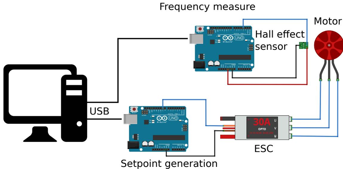
Figure 6.8 – Test bench ESC driver + motor.
