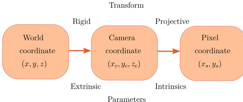
Figure 2.5 – Relation between extrinsic and intrinsic parameters.
