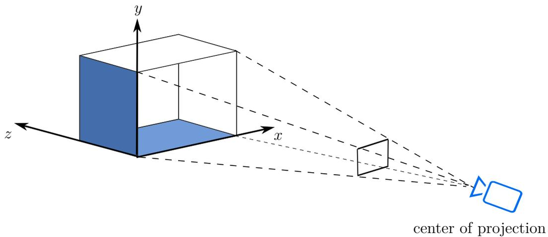
Figure 2.7 – Perspective projection of a cube.
