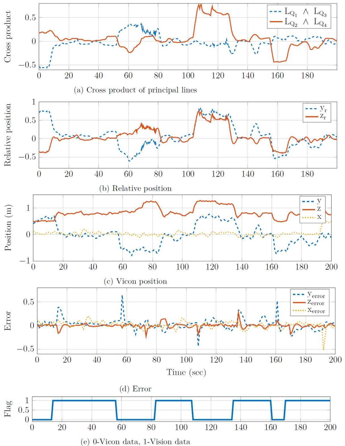
Figure 6.17 – Stabilization using vehicle-Vicon system and Babylon 3D.
