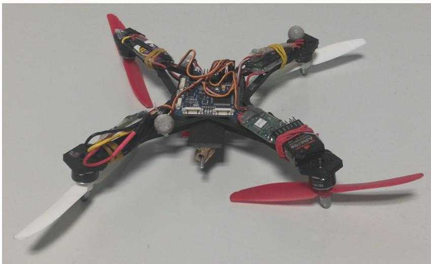
Figure 6.4 – Mosca quadrotor developed at GIPSA-LAB.
