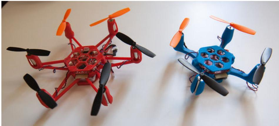
Figure A.1 – Flexbot platforms, hexa-rotor and qua-drotor.
