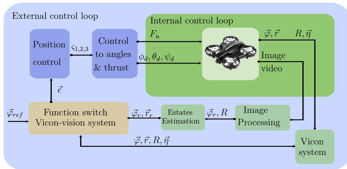
Figure 5.6 – Quadrotor system stabilization strategy: Real video scheme.
