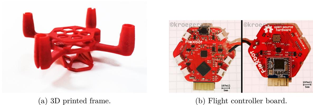
Figure A.2 – 3D printed frame of the Flexbot quad-rotor and the flight controller board.
