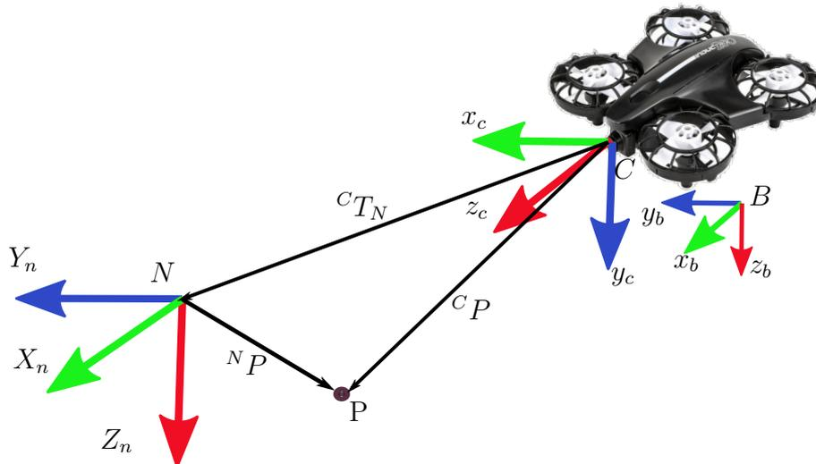
Figure 3.6 – The camera model system has its center of projection on the lens, which is the camera reference frame  $\mathbf{C}$ . The  $z_c$ -axis is going outwards to the optical axis,  $x_c$ -axis to the right and the  $y_c$ -axis downwards.
