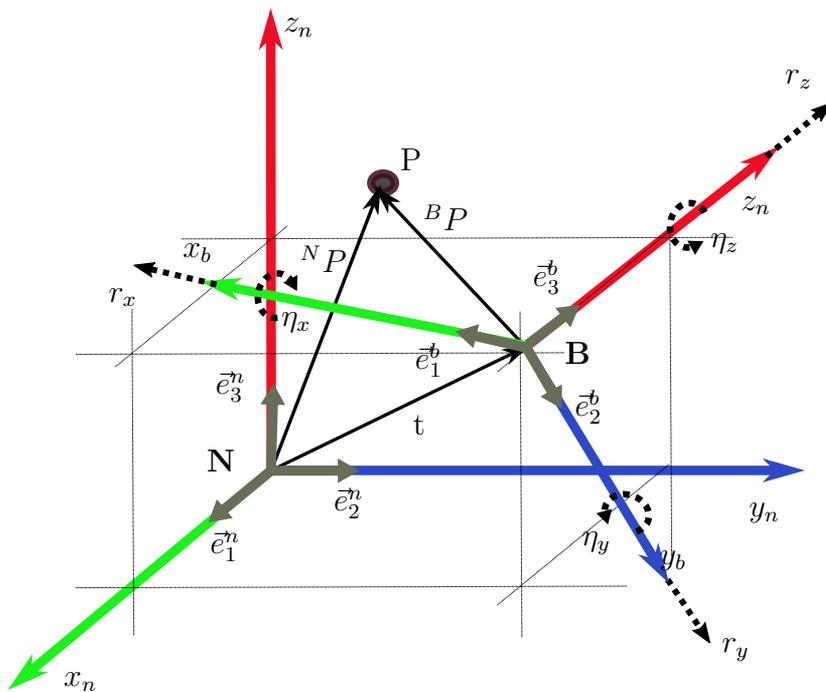
Figure 3.2 – Two coordinate frames, a point  $p$  whose coordinates can be given with respect to frame  $\mathbf{B}$  or  $\mathbf{N}$ .
