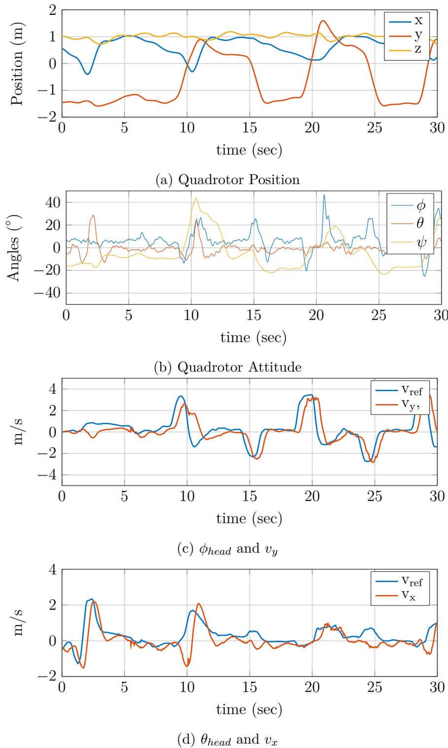
Figure B.3 – Backstepping Velocity Control with head movement
