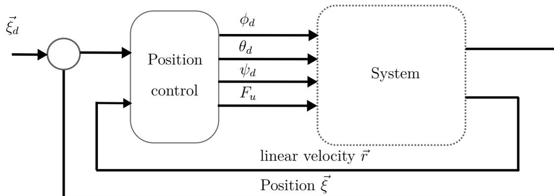
Figure 5.3 – Position control scheme.
