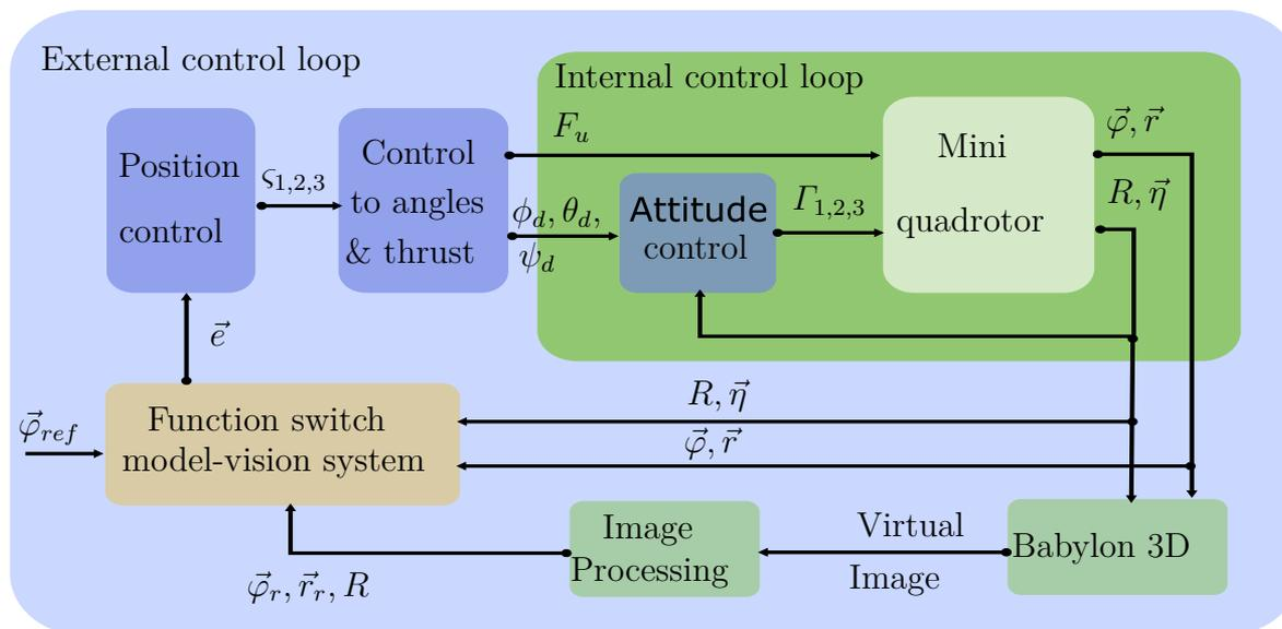
Figure 5.4 – Quadrotor system navigation strategy: Simulation scheme.
