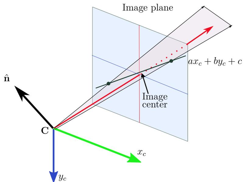
Figure 2.2 – Line projection and normal vector representation.
