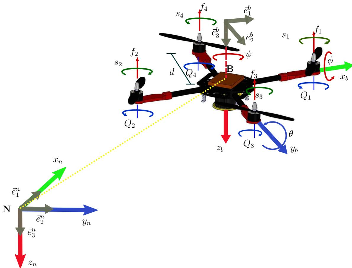
Figure 3.4 – Scheme of the quadrotor configuration: inertial frame  $\mathbf{N}[\vec{e}_1^n, \vec{e}_2^n, \vec{e}_3^n]$ , the body fixed frame  $\mathbf{B}[\vec{e}_1^b, \vec{e}_2^b, \vec{e}_3^b]$ , the  $f_i$  force on each motor, angular velocity of the motors  $s_i$  and the reaction torques  $Q_i$ .
