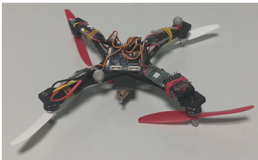
Figure 6.4 – Mosca quadrotor developed at GIPSA-LAB.
