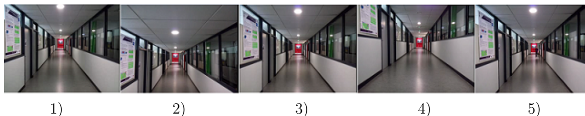
Figure 4.13 – Pictures with a camera in the middle of a corridor with up and down movements. In this sequence: Starting from left side 1) stay at the middle, 2) move up, 3) returns to the middle, 4) move down and 5) returns to the middle.
