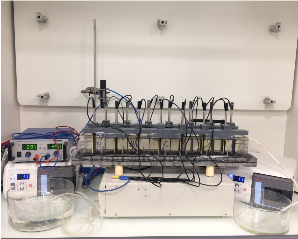
Fig. 50: The pilot reactor of 1.7 L and the whole set up.
