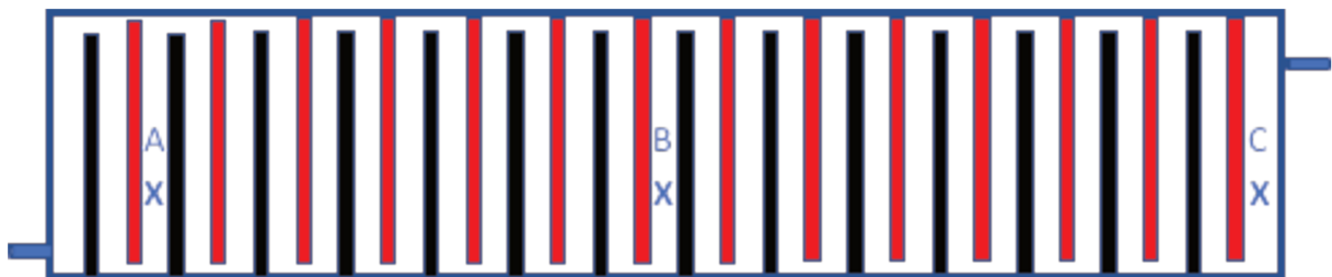
Fig. 48: Schematic representation of the pilot in the configuration with 28 electrodes with the position of sampling
