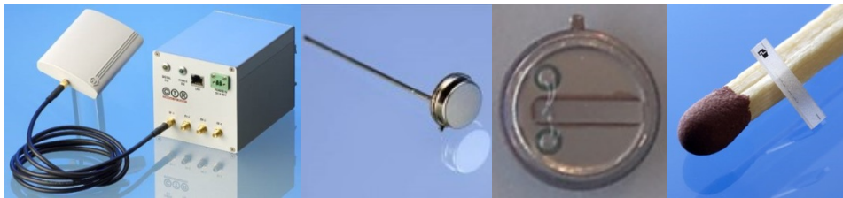
Figure 1.14 Pictures of the sensors developed at CTR. From left to right are presented, a reader, a packaged SAW sensor with its antenna, the same sensor with its package opened and a sensor chip. The reader was developed at CTR; it is meant to interrogate SAW delay-lines working in the ISM band at 2.45GHz. The interrogation principle is based on the Frequency Sweep of Continuous Waves (FSCW).
