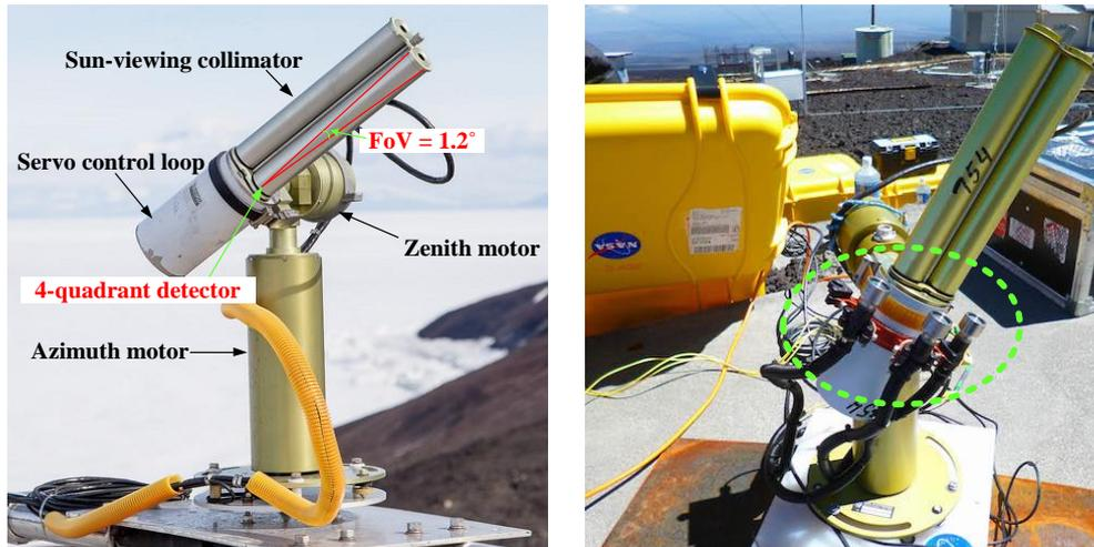
**Figure 2.3** *left*: CSPHOT sun-photometer; *right*: sunlight collection optics (circled by *green dotted line*) installed on the CSPHOT sun-photometer, involved in NASA's near-IR-LHR setup.
