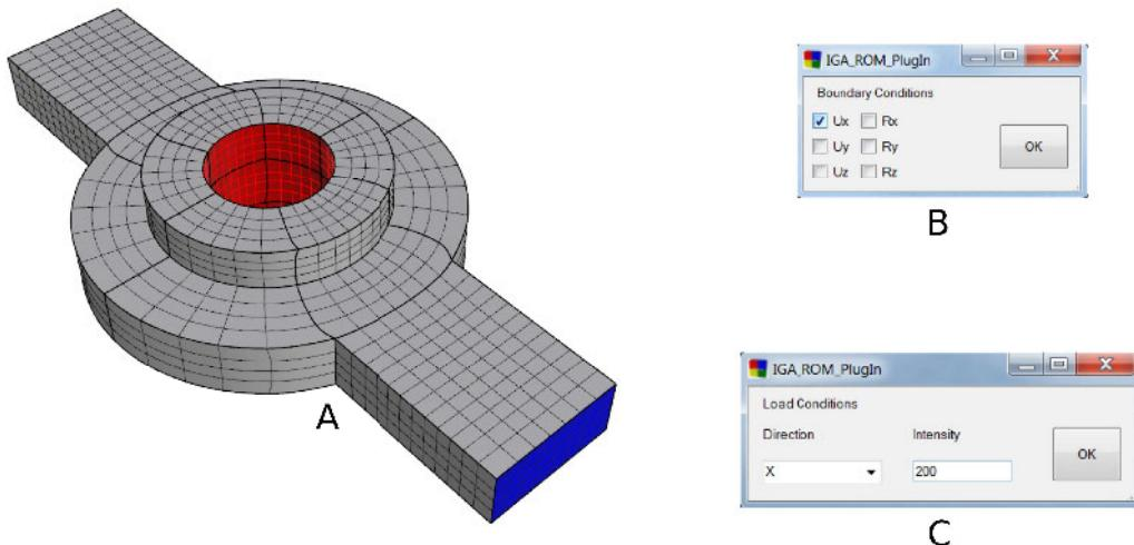
**Figure B.4:** Inputs of a volumetric isogeometric model in order to build pre-processing files. Conditions are settled directly into Rhinoceros 5. (A) Boundary conditions and loads applied to the trivariate isogeometric model boundary surfaces. (B) Blue surface holding boundary conditions. Red surfaces are subject to loads in (C).
