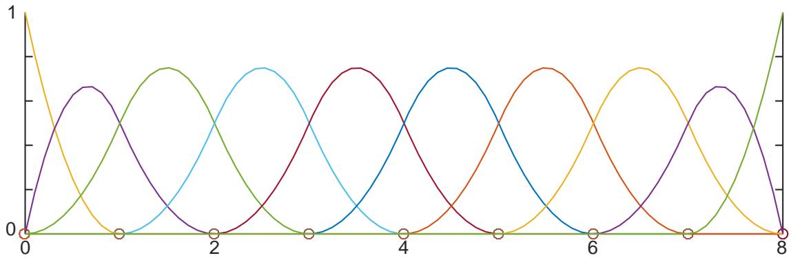
**Figure 1.5:** Quadratic basis functions generated by the knot vector  $\Xi$ . All quadratic basis functions generated by the knot vector  $\Xi = \{0, 0, 0, 1, 2, 3, 4, 5, 6, 7, 8, 8, 8\}$ . Each individual basis function can be described using a local knot vector of  $p + 2$  knots each. Picture from [Occelli 2018].
