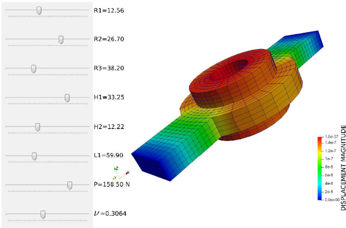
**Figure 7.14:** Seal reduced order model real-time evaluation. A 9-dimensional manifold built by kriging tools is evaluated to find preponderant coefficients attached to the first 50 modes. Isogeometric elements are sampled with one hexahedron per element for viewing purposes in Paraview. Used range of parameters is detailed in Table 7.2.
