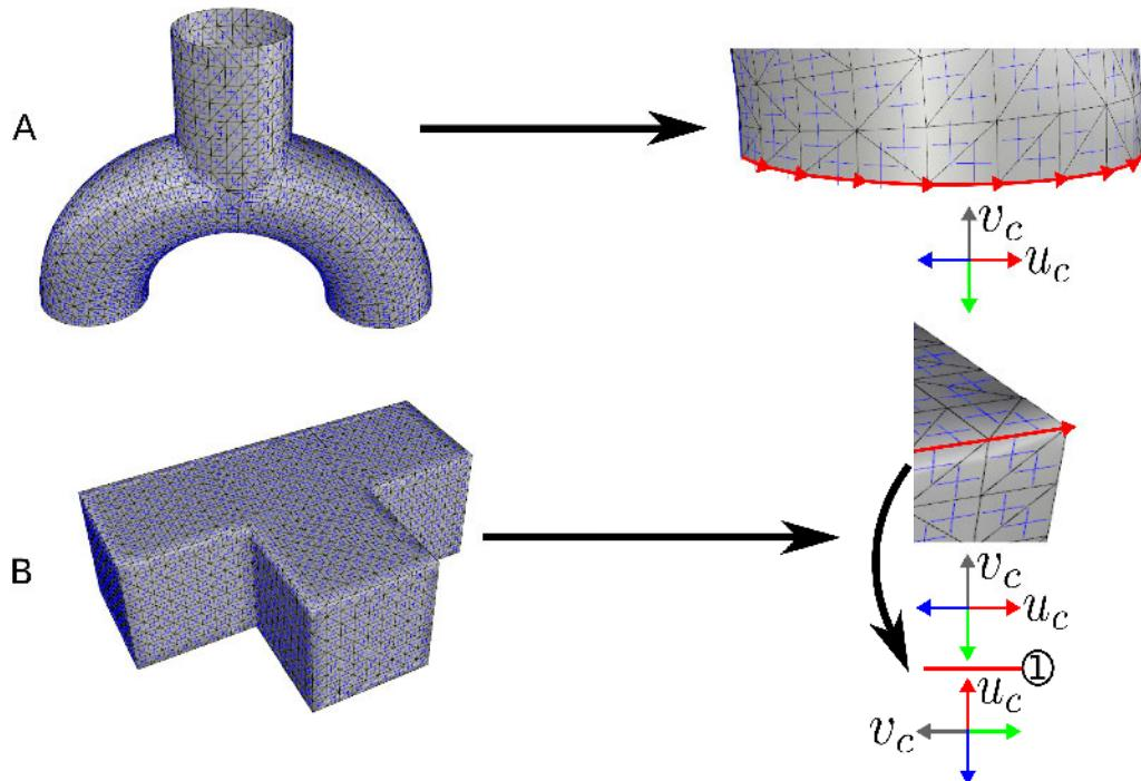
**Figure 4.9:** Cross field geometrical design. (A) Boundary red constraints interpolation. (B) Sharp edges red constraints interpolation. Across these sharp edges, the period jump is equal to 1, because of the  $s = \frac{1}{4}$  singularity held by the corner.
