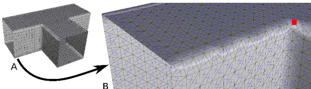
**Figure 4.6:** Cross field topological design with sharp features. (A) Input triangulated surface. (B) Generated cross field which does not understand the geometrical features of the mesh. The turning number around the red singularity remains consistent.
