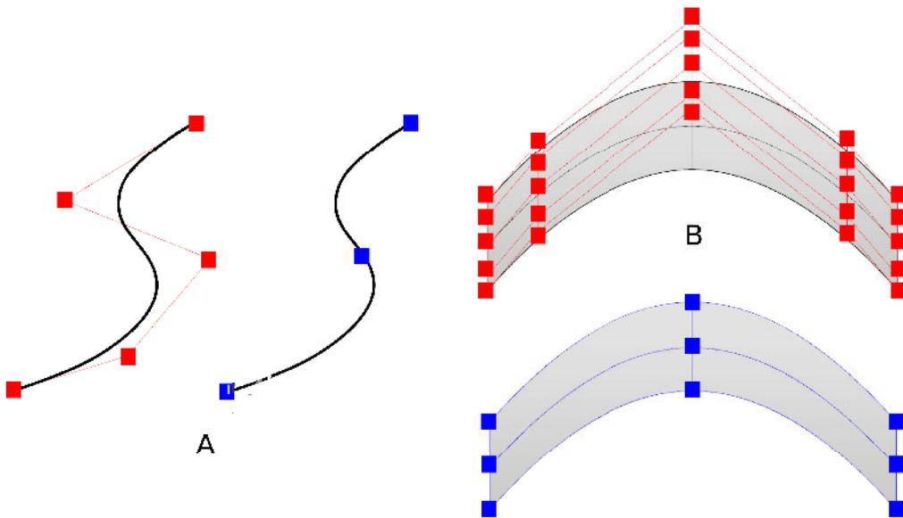
**Figure 1.6:** Cubic B-spline curve and surface. (A) A B-Spline curve with knot vector  $\Xi = \{0, 0, 0, 0, 1, 2, 2, 2, 2\}$ . (B) A B-Spline surface with knot vector  $\Xi = \{0, 0, 0, 0, 0, 1, 2, 2, 2, 2\}$  and  $\mathcal{H} = \{0, 0, 0, 0, 1, 2, 2, 2, 2, 2\}$ . Control points are depicted in red, whereas physical knot locations are in blue.
