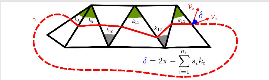
**Figure 4.4:** Discrete holonomy on triangulated meshes for a cycle  $\gamma$ . We observe an angle defect  $\delta$  between  $\mathcal{V}_s$  and  $\mathcal{V}_e$  using the classical Levi-Civita connection along a cycle  $\gamma$  to transport a vector  $\mathcal{V}_s$ .
