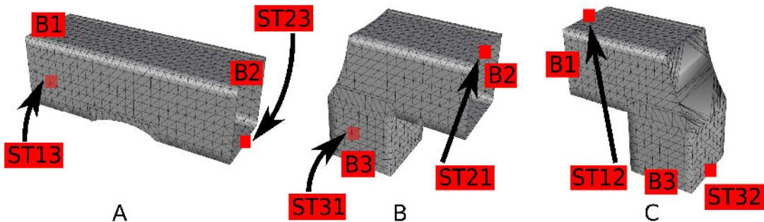
**Figure 3.6:** Boundary seed points computation. Temporary patches  $P_{T_3}$ ,  $P_{T_1}$  and  $P_{T_2}$  respectively in (A), (B) and (C). Using an approach close to circular conformal mapping of [Zeng et al. 2009a], temporary seed points  $s_{T_k}$  are determined into each respective patch  $P_{T_k}$ .
