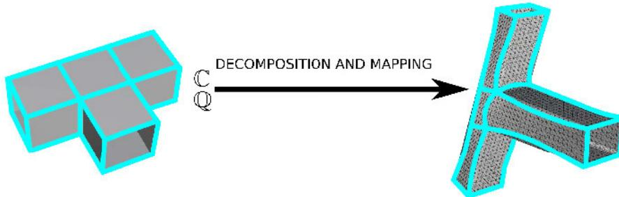
**Figure 3.4:** Cuboid configuration mapping onto a triangulated geometry yielding to a cuboid decomposition of the mesh.  $\mathbb{C}$  and  $\mathbb{Q}$  are both surface entities possibly with boundaries.  $\mathbb{C}$  holds additional properties to build a volume due to its cuboid structure.
