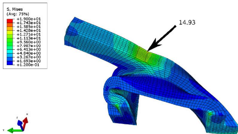
**Figure 7.6:** ABAQUS Von-Mises stress results on the unremeshed half-seal part. Notice that values are averaged on hexahedral elements nodes and the color scale is interpolated at scalar values embedded on these nodes. The Von-Mises value of 14.93 is not averaged and resides at a physical Gauss point.
