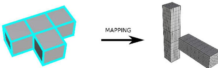
**Figure 7.9:** Volumetric isogeometric parameterization of the pant part. It is a genus-0 geometry with sharp features. Euler characteristic is  $\chi = -1$  for the associated mesh  $M$  with 3 boundaries. We apply the same parameterization among all members of the population to obtain isotopological comparable isogeometric meshes.
