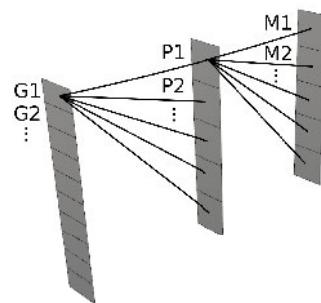
**Figure 7.8:** Parameters tensorial product. For each geometrical cases  $G$ , we associate all loading cases  $P$ . Each loading parameter is then combined with all mechanical cases  $M$ . This method resulting in  $\dim(G) \times \dim(P) \times \dim(M)$  snapshots.
