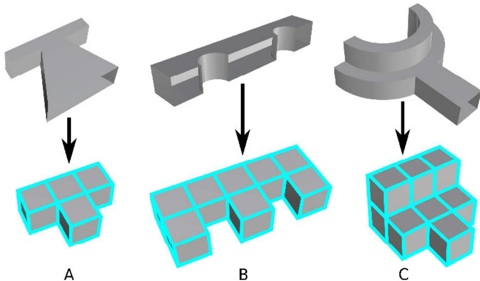
**Figure 3.11:** Cuboid configuration templates C. To understand all the features of a CAD model, a specific cuboid configuration has to be applied for mapping purposes. (A) Represents the simplest cuboid configuration C for a pant. (B) Configuration C with 8 cuboids. (C) Configuration C with 10 cuboids.
