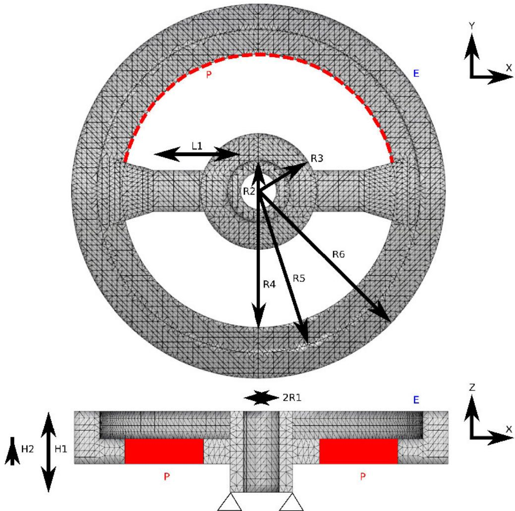
**Figure 7.16:** Wheel part distribution of parameters. 9 geometrical parameters are settled. 1 load parameter  $P$  is applied and Young's modulus  $E$  is devoted to be a mechanical parameter. We use a constant Poisson's ratio  $\nu = 0.3$ . Loads and boundary conditions are distributed on concerned nodes.
