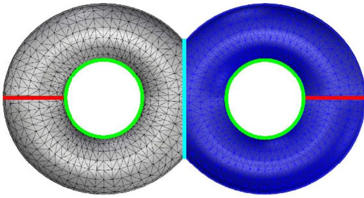
**Figure 2.9:** Pants decomposition of a double torus mesh computed from a CAD model by our IGA\_ROM PlugIn (see Appendix B). A double torus is a genus-2 surface without boundary and has Euler characteristic  $\chi = 2 - 2g - b = -2$ . Pants decomposition provides two pants (gray and blue meshes) by cutting along handle loops and using symmetry (symmetry loop is depicted in cyan). Homology basis is composed by two handle loops and two tunnel loops respectively depicted in red and green.
