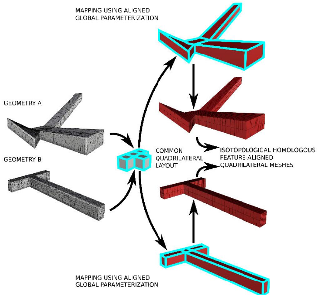
**Figure 1.12:** The MEG-IsoQuad strategy. Building isotopological homologous feature-aligned quadrilateral meshes from triangulated meshes with the same topology. Resulting isotopological meshes have non-uniform isotropy. Quadrilateral meshes have been computed by our IGA-ROM PlugIn (see Appendix B).
