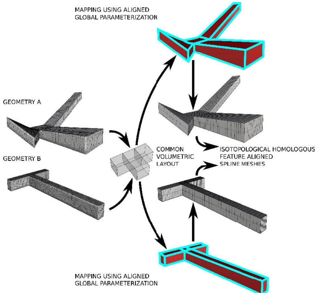
**Figure 1.14:** The **MEG-IsoHex strategy**. Building isotopological homologous feature-aligned hexahedral or spline meshes from triangulated meshes with the same topology. Resulting isotopological meshes have non-uniform isotropy. Trivariate spline meshes have been computed by our IGA-ROM PlugIn (see Appendix B).
