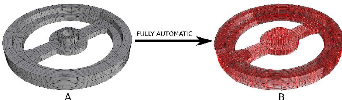
**Figure B.2:** Wheel fully automatic trivariate isogeometric parameterization. (A) Surfaces with required properties from CAD. (B) Computed trivariate parameterization. Boundary surfaces of the parameterization are represented in semi-transparent: color could be different depending on the normal orientation. CAD to isogeometric analysis suitable model is achieved in 15 seconds.
