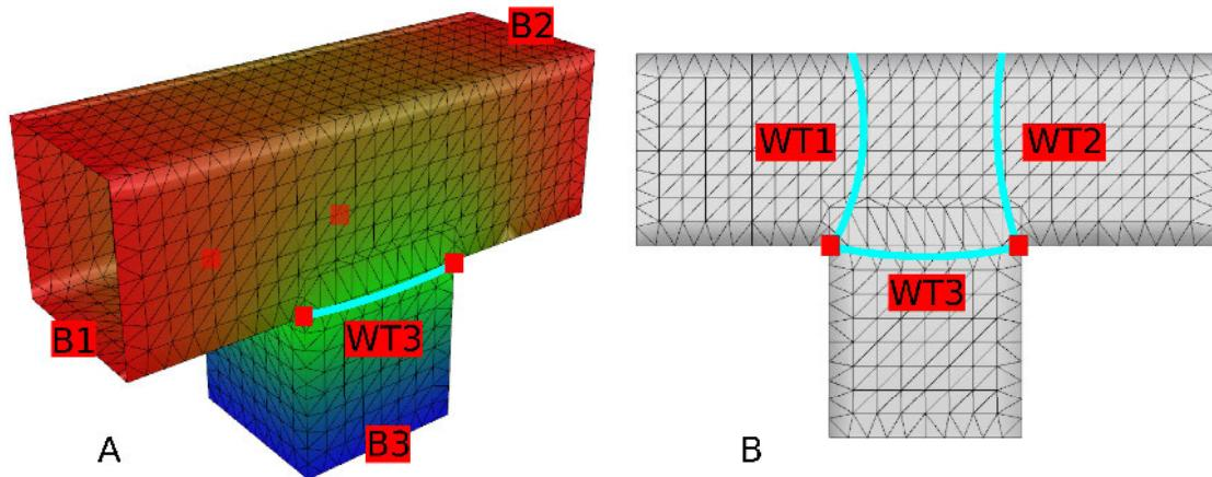
**Figure 3.5:** Temporary cutting curves generation. (A) Discrete harmonic function  $f_3$ . Blue color represents parametric values close to 0, red ones are close to 1. Using a set  $C$  of  $n_c$  sharp cutting points,  $f_2$  and  $f_1$ , the three temporary cutting curves are computed in (B).
