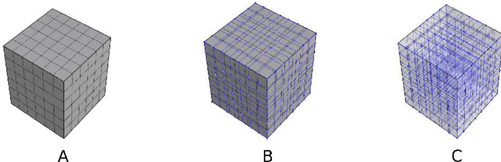
**Figure 7.1:** Hexahedral sampling method from B-Spline surfaces of degree 2. (A) 6 compatible B-Spline surfaces that bound a volume. Black lines delimit surfaces elements. (B) 6 quadrilateral meshes evaluated at physical positions of parametric values contained in vectors  $\mathcal{U}_q$  and  $\mathcal{V}_q$  of Equation (7.1) (quadrilateral meshes and points are depicted in blue). (C) Blue hexahedral patch computed using Coon's interpolation.
