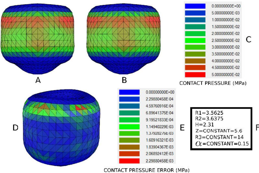
**Figure 5.17:** Web deployment reduced order model demonstrator validation. (A) Reduced order model evaluation constructed with a DOE of 50 snapshots, using parameters in (F). (B) Snapshot with parameters in (F) of the second DOE composed by 20 snapshots. (C) Pressure contact color scale for (A) and (B). (D) Pressure contact error between (A) and (B) using color scale (E).
