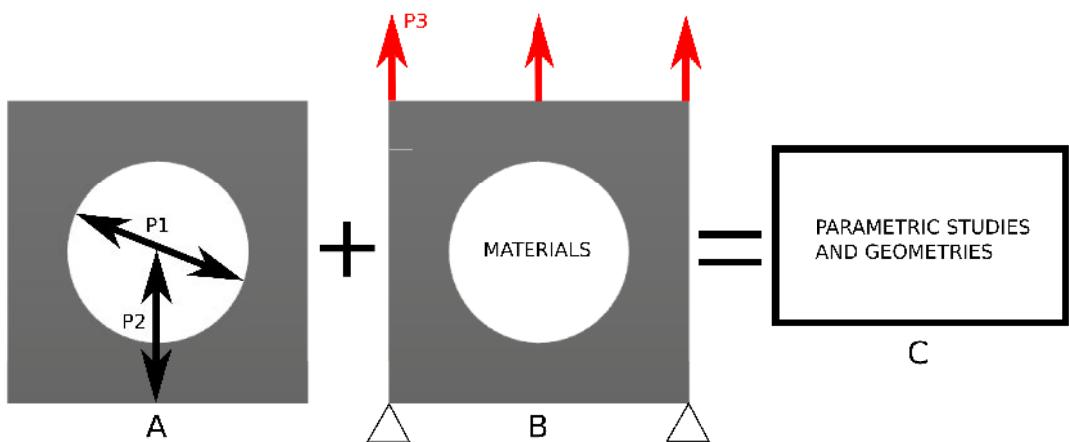
**Figure 1.8:** Parametric models generation. Reduced order modeling is a well-suited tool for these designing pipelines. (A) A feature based parametric design done in industries. (B) Applying loading parameters, boundary conditions and material properties. (C) Parametric studies and geometries resulted from (A) and (B).
