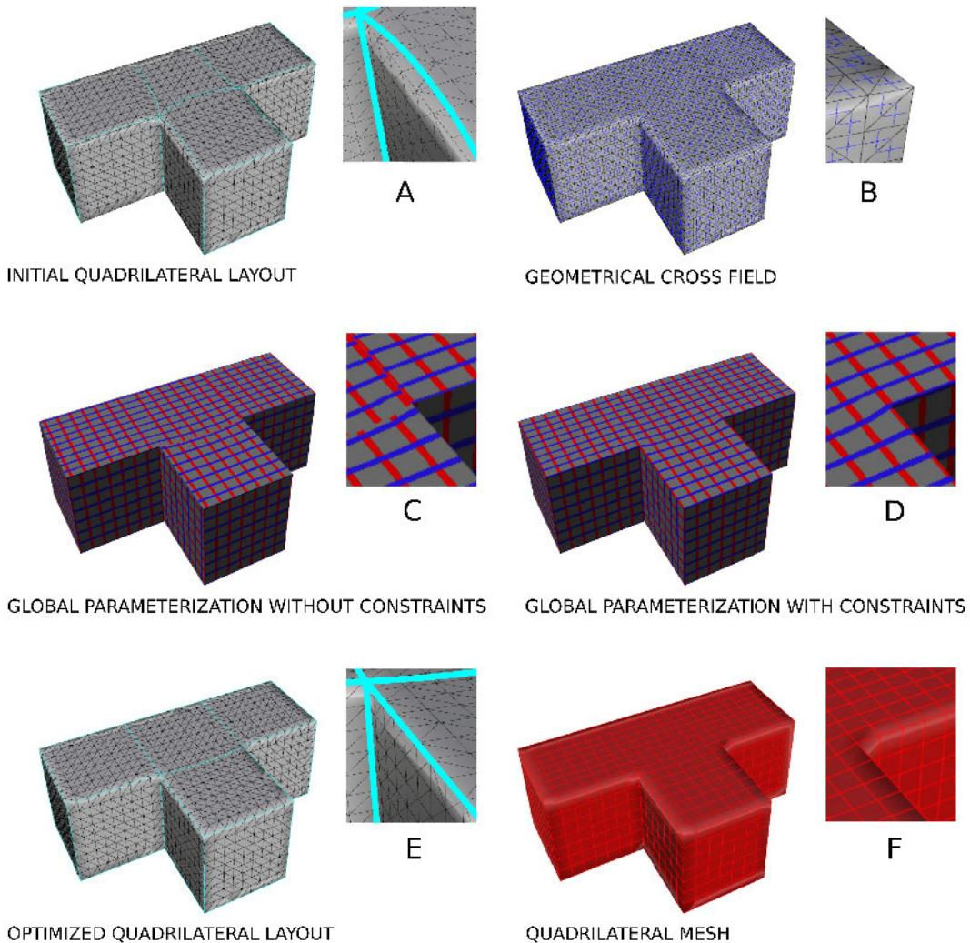
**Figure 4.12:** Aligned global parameterization worflow summary from geometry-feature-aware pants-to-cuboid decomposition. (A) Initial quadrilateral layout  $\mathbb{Q}$ . (B) Geometrical cross field. (C) Aligned global parameterization without constraints. (D) Aligned global parameterization with constraints. (E) Optimized quadrilateral layout embedding. (F) Extracted quadrilateral mesh.
