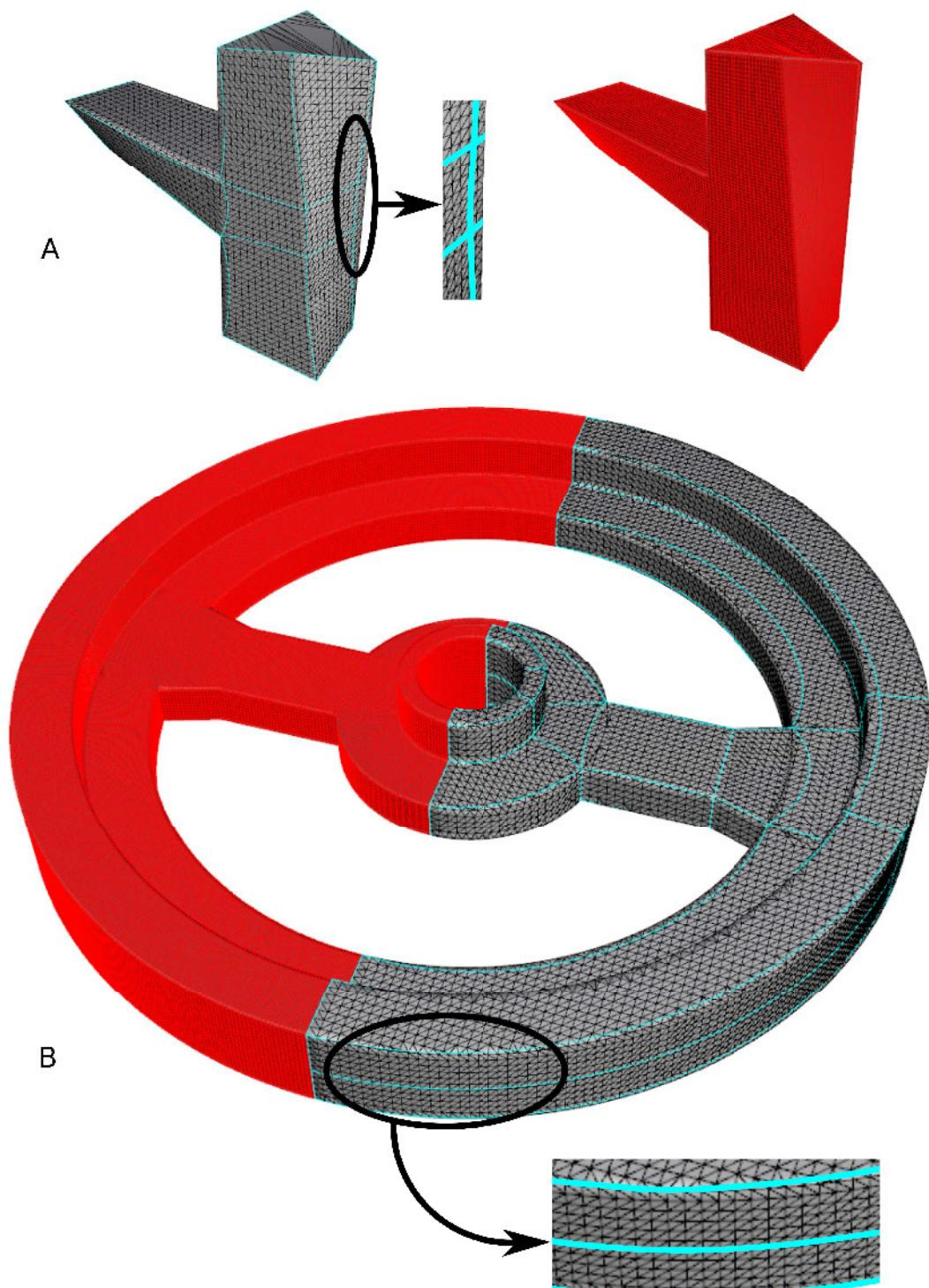
**Figure 4.13:** Mechanical quadrilateral mesh examples. (A) A pant part quadrilateral mesh with its feature-aware cuboid decomposition. (B) Symmetric wheel part quadrilateral mesh obtained by locating high valence nodes on curved areas.
