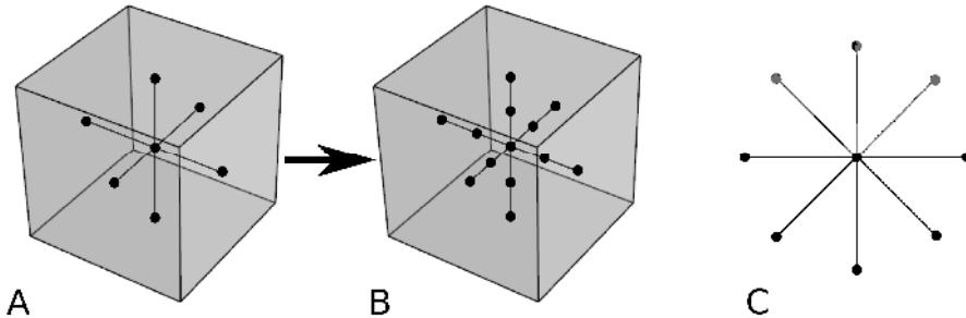
**Figure 5.5:** Snapshots sampling with a sparse grid technique. (A) Level 1 sparse grid of a 3-dimensional parameter space. (B) First refinement of the level 1 sparse grid. (C) 2D representation of a level 1 sparse grid of a 4-dimensional parameter space.
