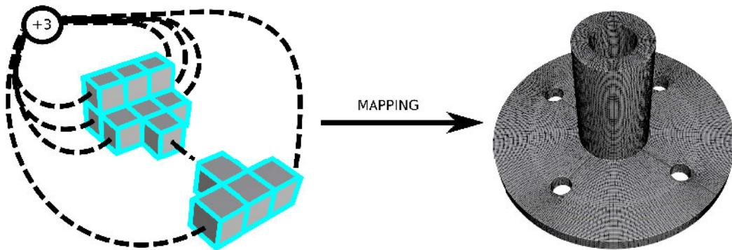
**Figure 5.12:** Quadrilateral mesh parameterization of the casting part. We apply the same parameterization among all members of the population to obtain isotopological comparable quadrilateral meshes.
