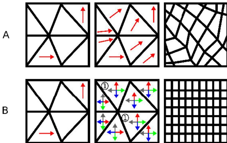
**Figure 4.8:** Cross field interpolation. (A) Sparse directions interpolation with a standard vector field. Parameterized mesh is not a suitable result for our objectives. (B) By using a cross field, i.e., a set of 4 directions, the resulting parameterized quadrilateral mesh as a natural expected geometry. Notice the period jump of 1, ensuring that the first red direction of the cross field match with given constrained directions.
