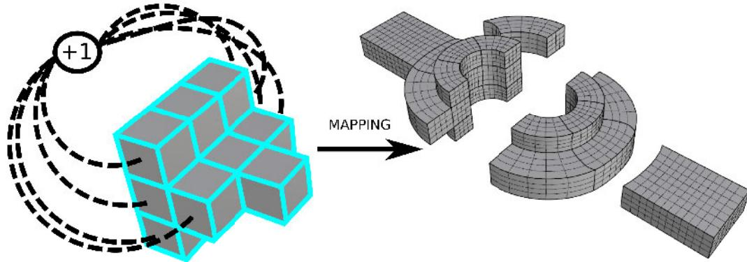
**Figure 7.12:** Volumetric isogeometric parameterization of the seal part. It is a genus-1 geometry with sharp features. Euler characteristic is  $\chi = 0$  for the associated closed mesh  $M_c$ . We apply the same parameterization among all members of the population to obtain isotopological comparable isogeometric meshes.
