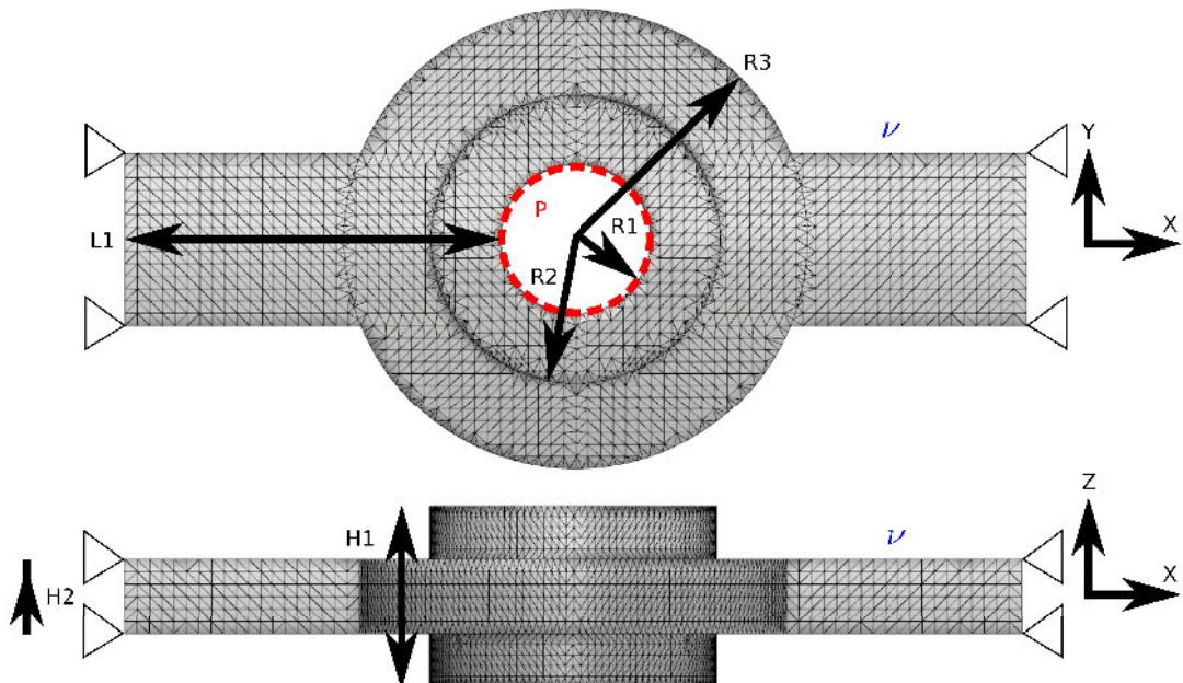
**Figure 7.13:** Seal part distribution of parameters. 6 geometrical parameters are settled. 1 load parameter  $P$  is applied and Poisson's ratio  $\nu$  is devoted to be a mechanical parameter. We use a constant Young's modulus  $E = 210$  GPa. Loads and boundary conditions are distributed on concerned nodes.
