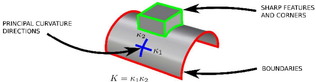
**Figure 4.7:** Relevant geometrical features which could be used for cross field interpolation. Sharp corners, boundaries and principal curvature directions refer to a certain global topological information embedded on the geometry. The Gauss-Bonnet theorem states the link between geometry and topology.
