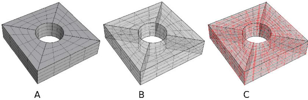
**Figure 6.10:** Trivariate B-Spline volume construction from B-Spline surfaces. (A) B-Spline surfaces extracted thanks to the parameterization. (B) Reconstructed missing interior surfaces needed for the trivariate parametric domain. (C) Interpolated trivariate isogeometric control lattice (depicted in red).
