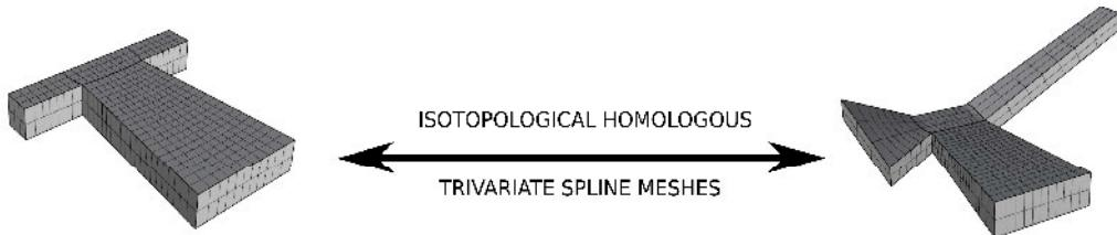
**Figure 1.13:** Isogeometric and hexahedral meshes problematic for ROMs of different meshes with the same topology. Problematic is given as an answer using trivariate splines. To overcome this issue, a proposed strategy is given in Strategy 1.2. Trivariate spline meshes have been computed by our IGA\_ROM PlugIn (see Appendix B).
