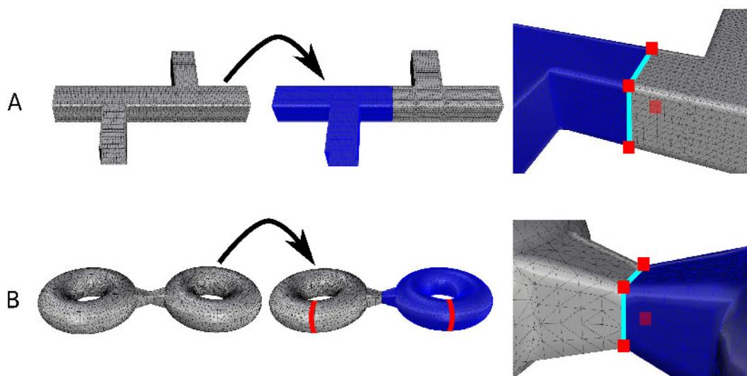
**Figure 3.2:** Geometry-aware pants decomposition with sharp points. (A) Double T is decomposed into pants using 4 sharp points given by the user or determined automatically. (B) A 2-torus pants decomposition passing through sharp points. Notice that using shortest length loops, the result will be the same for (B).
