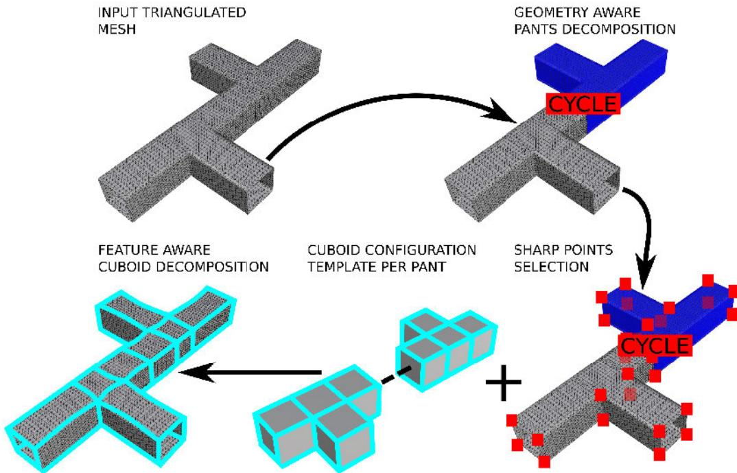
**Figure 3.9:** Smart model decomposition overview for mechanical applications. Starting with a triangulated surface, we decompose into a set of topological pants understanding the geometry. Afterwards, depending on the features embedded in the input mesh, cuboid configuration templates per pant are chosen. These templates are then mapped back into the surface mesh yielding to a feature-aware cuboid decomposition.
