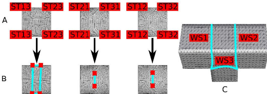
**Figure 3.7:** Sharp cutting curves generation. (A) The three temporary unit square maps  $U_{T_3}$ ,  $U_{T_1}$  and  $U_{T_2}$  (left to right). (B) Partial line inverse mapping using sharp cutting points in  $C$  performed in  $U_{T_3}$ ,  $U_{T_1}$  and  $U_{T_2}$  (left to right). (C) Computed sharp cutting curves  $W_{S_1}$ ,  $W_{S_2}$  and  $W_{S_3}$ .
