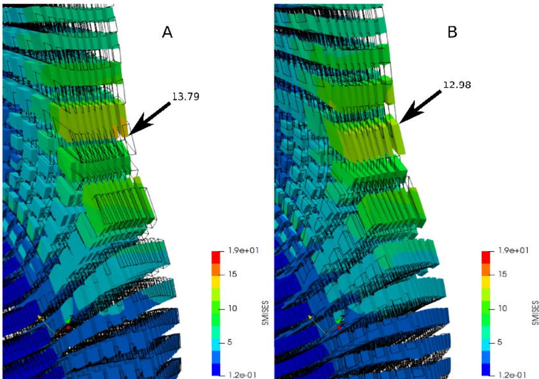
**Figure 7.5:** Details of Von-Mises stress comparison at Gauss points. For each hexahedral element, we build an associated linear hexahedral element which geometry is described by its related Gauss points. (A) Stress for the unremeshed case at  $t = 1$ . Elements made by Gauss points of the remeshed part are depicted in black wireframe. (B) Stress for the remeshed case at  $t = 1$ . Elements made by Gauss points of the unremeshed part are depicted in black wireframe.
