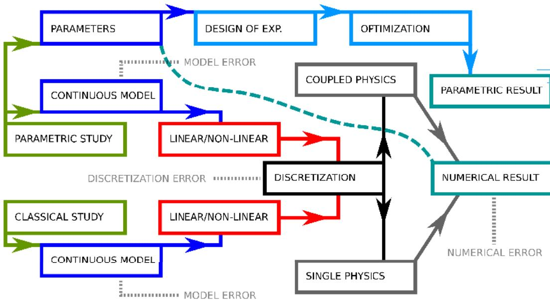
**Figure 1.3:** Increasing model complexity for more realistic simulations. Starting from a classical study or a parametric one, numerous additional stages with expensive computational costs can be added depending on the physics. Numerical result is obtained after a few minutes for simple problems or months for FSI (Fluid Structure Interactions) studies. Such nested steps are subject to several errors: modeling, discretization and numerical errors.
