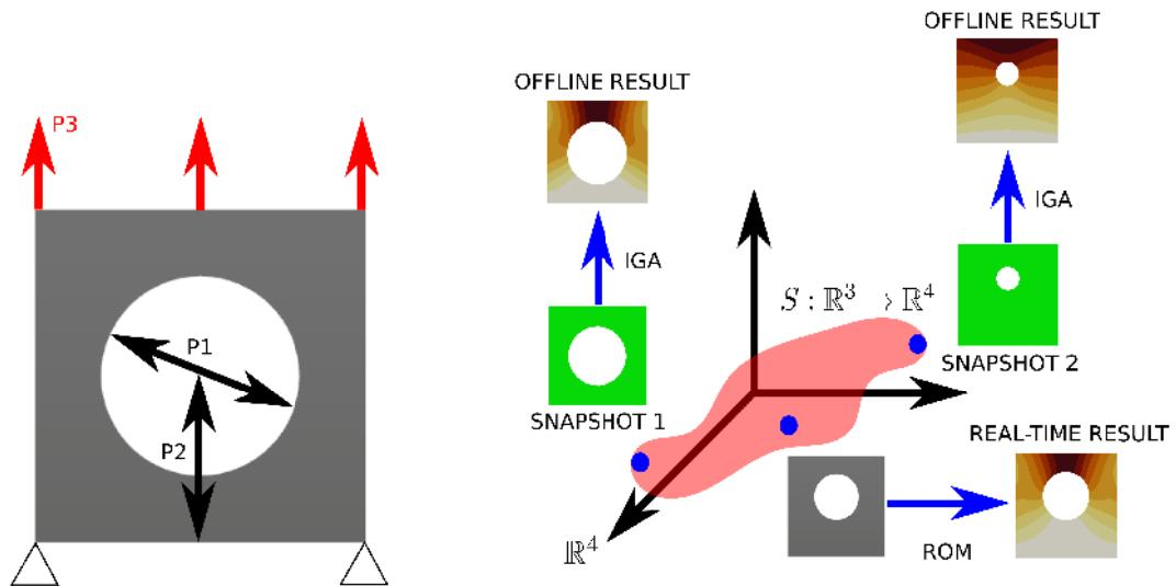
**Figure 7.7:** Reduced order model building and evaluation for a plate with one hole. Snapshots are calculated using isogeometric analysis.  $P_1$  and  $P_2$  are geometrical parameters defining respectively the diameter and the position of the hole along his height.  $P_3$  is a loading parameter. Response surfaces  $S$  are embedded in 4-dimensional space. There are as many surfaces as there are modes in the reduced basis.
