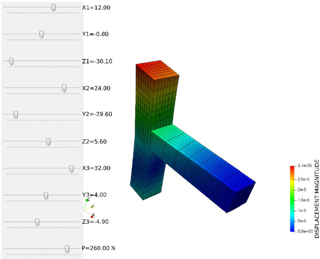
**Figure 7.11:** Pant reduced order model real-time evaluation. A 10-dimensional manifold built by kriging tools is evaluated to find preponderant coefficients attached to the first 60 modes. Isogeometric elements are sampled with one hexahedron per element for viewing purposes in Paraview. Used range of parameters is detailed in Table 7.1.
