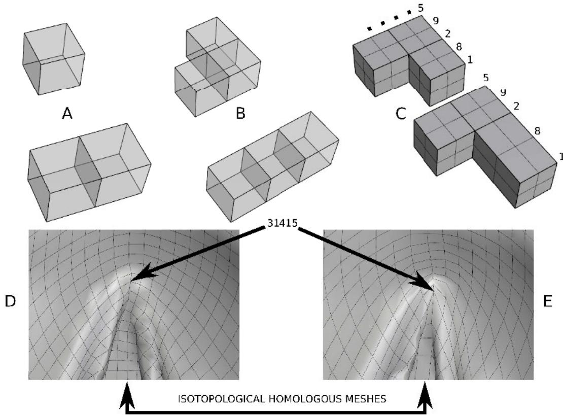
**Figure 6.8:** Isotopological homologous properties of volumetric meshes. (A) Non-isomorphic volumetric layouts. (B) Isomorphic layouts with a discontinuous mapping function. (C) Isotopological trivariate isogeometric meshes. (D) and (E) are representing the homologous concept for an aortic valve using quadrilateral meshes.
