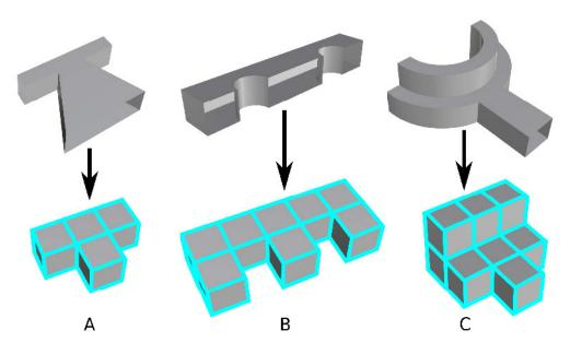
**Figure 3.11:** Cuboid configuration templates  $\mathbb{C}$ . To understand all the features of a CAD model, a specific cuboid configuration has to be applied for mapping purposes. (A) Represents the simplest cuboid configuration  $\mathbb{C}$  for a pant. (B) Configuration  $\mathbb{C}$  with 8 cuboids. (C) Configuration  $\mathbb{C}$  with 10 cuboids.
