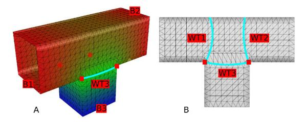
**Figure 3.5:** Temporary cutting curves generation. (A) Discrete harmonic function  $f_3$ . Blue color represents parametric values close to 0, red ones are close to 1. Using a set C of  $n_c$  sharp cutting points,  $f_2$  and  $f_1$ , the three temporary cutting curves are computed in (B).
