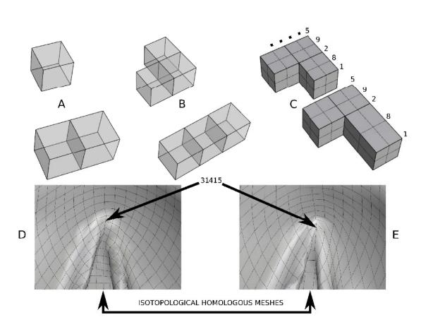
**Figure 6.8:** Isotopological homologous properties of volumetric meshes. (A) Nonisomorphic volumetric layouts. (B) Isomorphic layouts with a discontinuous mapping function. (C) Isotopological trivariate isogeometric meshes. (D) and (E) are representing the homologous concept for an aortic valve using quadrilateral meshes.
