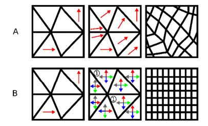
Figure 4.8: Cross field interpolation. (A) Sparse directions interpolation with a standard vector field. Parameterized mesh is not a suitable result for our objectives. (B) By using a cross field, i.e., a set of 4 directions, the resulting parameterized quadrilateral mesh as a natural expected geometry. Notice the period jump of 1, ensuring that the first red direction of the cross field match with given constrained directions.
