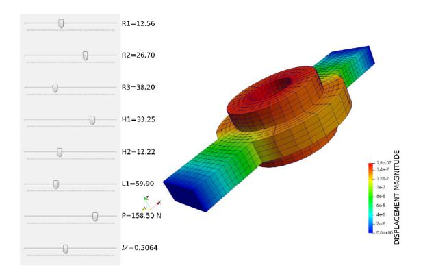
Figure 7.14: Seal reduced order model real-time evaluation. A 9-dimensional manifold built by kriging tools is evaluated to find preponderant coefficients attached to the first 50 modes. Isogeometric elements are sampled with one hexahedron per element for viewing purposes in Paraview. Used range of parameters is detailed in Table 7.2.
