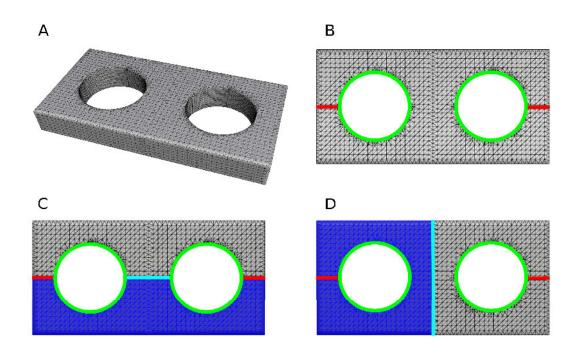
**Figure 3.1:** Genus-2 plate pants decomposition. (A) Input triangulated surface. (B) Surface with its handle and tunnel loops, depicted in red and green respectively. Pants decomposition using loops with shortest distance (C) and with symmetry (D).
