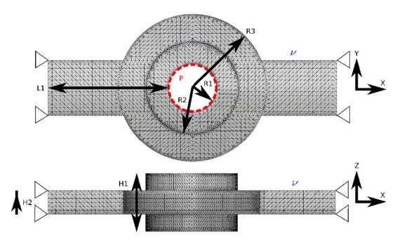
Figure 7.13: Seal part distribution of parameters. 6 geometrical parameters are settled. 1 load parameter P is applied and Poisson's ratio  $\nu$  is devoted to be a mechanical parameter. We use a constant Young's modulus E = 210 GPa. Loads and boundary conditions are distributed on concerned nodes.
