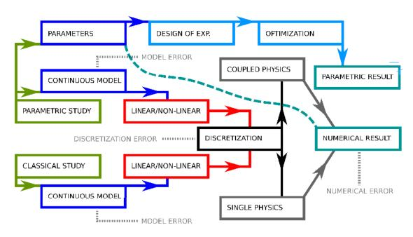
**Figure 1.3:** Increasing model complexity for more realistic simulations. Starting from a classical study or a parametric one, numerous additional stages with expensive computational costs can be added depending on the physics. Numerical result is obtained after a few minutes for simple problems or months for FSI (Fluid Structure Interactions) studies. Such nested steps are subject to several errors: modeling, discretization and numerical errors.
