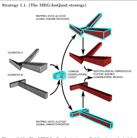
Figure 1.12: The MEG-IsoQuad strategy. Building isotopological homologous feature-aligned quadrilateral meshes from triangulated meshes with the same topology. Resulting isotopological meshes have non-uniform isotropy. Quadrilateral meshes have been computed by our IGA\_ROM PlugIn (see Appendix B).
