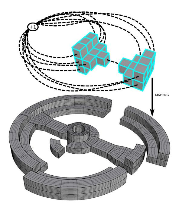
Figure 7.15: Volumetric isogeometric parameterization of the wheel part. It is a complex genus-3 geometry with sharp features. Euler characteristic is equal to  $\chi = -4$ , involving a decomposition in 4 pants. We apply the same parameterization among all members of the population to obtain isotopological comparable isogeometric meshes.
