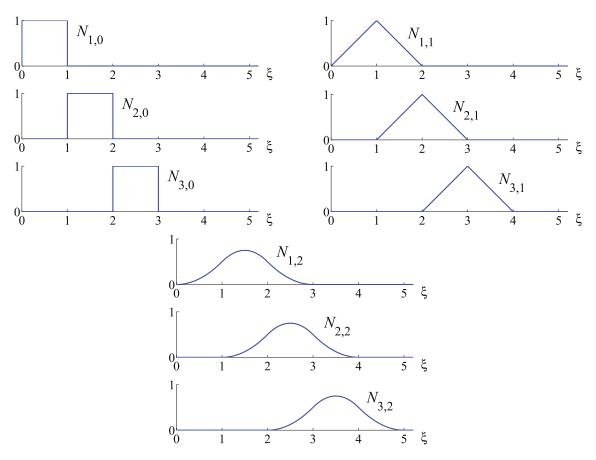
**Figure 1.4:** B-spline basis functions of order p = 0, 1 or 2 for a uniform knot vector  $\{0, 1, 2, 3, 4, \ldots\}$ . Picture from [Cottrell, Hughes, and Bazilevs 2009].
