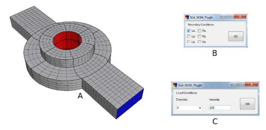
Figure B.4: Inputs of a volumetric isogeometric model in order to build preprocessing files. Conditions are settled directly into Rhinoceros 5. (A) Boundary conditions and loads applied to the trivariate isogeometric model boundary surfaces. (B) Blue surface holding boundary conditions. Red surfaces are subject to loads in (C).
