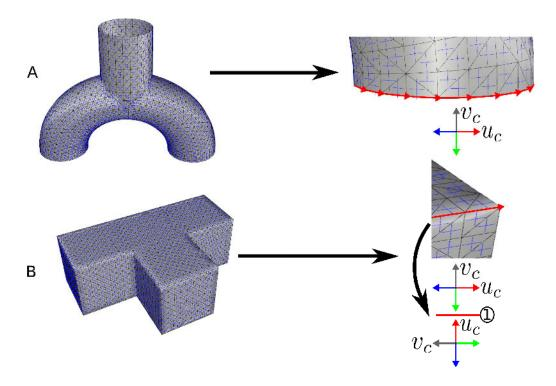
**Figure 4.9:** Cross field geometrical design. (A) Boundary red constraints interpolation. (B) Sharp edges red constraints interpolation. Across these sharp edges, the period jump is equal to 1, because of the  $s = \frac{1}{4}$  singularity holded by the corner.
