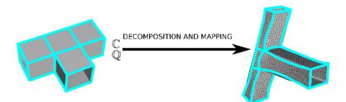
**Figure 3.4:** Cuboid configuration mapping onto a triangulated geometry yielding to a cuboid decomposition of the mesh.  $\mathbb{C}$  and  $\mathbb{Q}$  are both surface entities possibly with boundaries.  $\mathbb{C}$  holds additional properties to build a volume due to its cuboid structure.
