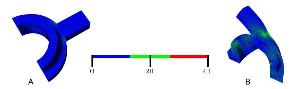
**Figure C.1:**  $\frac{3\pi}{2}$  Gaussian curvature element quality metric. Example is shown using meshes from Chapter 7. (A) Element quality for the half-seal undeformed shape. (B) Element quality for the associated deformed shape of (A) at the intermediate loading step, t = 0.5. Element quality has been computed by our IGA\_ROM PlugIn (see Appendix B).
