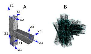
**Figure 5.9:** Geometrical snapshots generation of the pant part. (A) Zero reference of geometrical parameters in the attached local frames. (B) Feature-aware cuboid decomposition of all geometrical instances.
