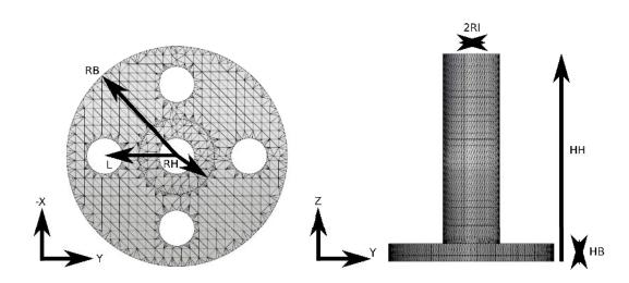
Figure 5.13: Casting part distribution of parameters. 6 geometrical parameters are settled.
