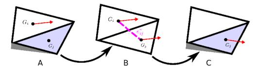
**Figure 4.2:** Levi-Civita connection using triangulated mesh faces. (A) Transporting a vector from face  $f_i$  to  $f_j$  of gravity centers  $G_i$  and  $G_j$  can be done as follows: (B) unfold the faces isometrically to a plane, parallel transport the vector along the oriented dual edge  $e_{ij}^*$  and then (C) fold back the face in its original configuration.
