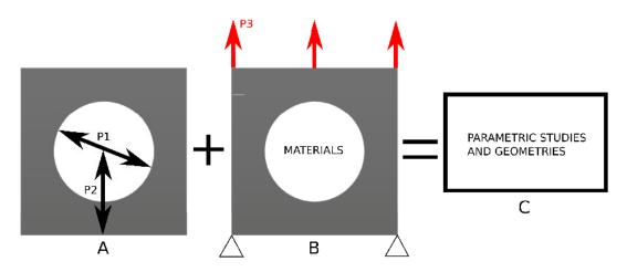
Figure 1.8: Parametric models generation. Reduced order modeling is a well-suited tool for these designing pipelines. (A) A feature based parametric design done in industries. (B) Applying loading parameters, boundary conditions and material properties. (C) Parametric studies and geometries resulted from (A) and (B).
