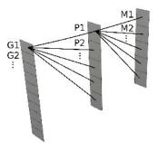
Figure 7.8: Parameters tensorial product. For each geometrical cases G, we associate all loading cases P. Each loading parameter is then combined with all mechanical cases M. This method resulting in dim  $(G) \times \dim(P) \times \dim(M)$  snapshots.
