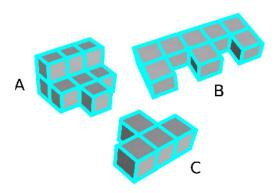
Figure 6.4: Genus-0 closed cuboid configuration  $\mathbb{C}_c$  examples with Euler characteristic  $\chi = 2$ . (A) Configuration with 28 nodes. (B) Configuration with 36 nodes. (C) Configuration with 20 nodes. These configurations are coming from Chapter 3.
