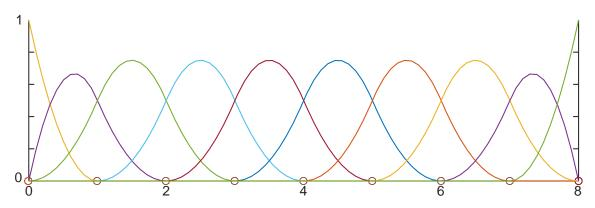
**Figure 1.5:** Quadratic basis functions generated by the knot vector  $\Xi$ . All quadratic basis functions generated by the knot vector  $\Xi = \{0, 0, 0, 1, 2, 3, 4, 5, 6, 7, 8, 8\}$ . Each individual basis function can be described using a local knot vector of p + 2 knots each. Picture from [Occelli 2018].
