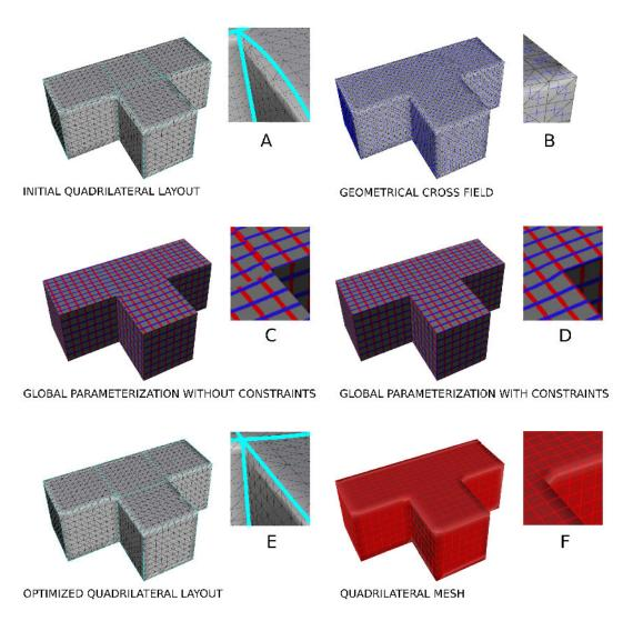
Figure 4.12: Aligned global parameterization worflow summary from geometry-feature-aware pants-to-cuboid decomposition. (A) Initial quadrilateral layout  $\mathbb{Q}$ . (B) Geometrical cross field. (C) Aligned global parameterization without constraints. (D) Aligned global parameterization with constraints. (E) Optimized quadrilateral layout embedding. (F) Extracted quadrilateral mesh.
