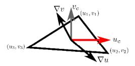
Figure 4.10: Global parameterization strategy using a geometrical cross field. We strive to find gradients  $\nabla u$  and  $\nabla v$  aligned to the first two parametric directions  $\mathcal{U}_c$  and  $\mathcal{V}_c$  of the cross field, by modifying parametric values (u, v) embedded in mesh vertices.
