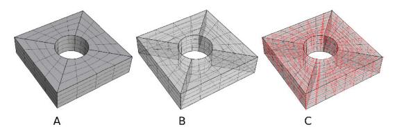
**Figure 6.10:** Trivariate B-Spline volume construction from B-Spline surfaces. (A) B-Spline surfaces extracted thanks to the parameterization. (B) Reconstructed missing interior surfaces needed for the trivariate parametric domain. (C) Interpolated trivariate isogeometric control lattice (depicted in red).
