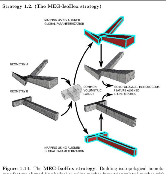
**Figure 1.14:** The **MEG-IsoHex strategy**. Building isotopological homologous feature-aligned hexahedral or spline meshes from triangulated meshes with the same topology. Resulting isotopological meshes have non-uniform isotropy. Trivariate spline meshes have been computed by our IGA\_ROM PlugIn (see Appendix B).
