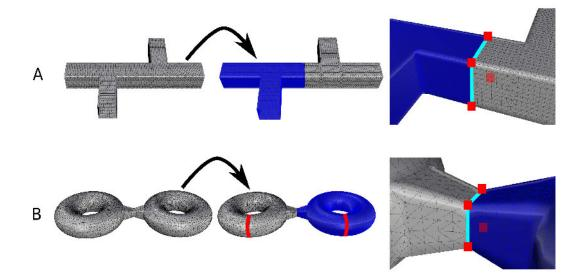
**Figure 3.2:** Geometry-aware pants decomposition with sharp points. (A) Double T is decomposed into pants using 4 sharp points given by the user or determined automatically. (B) A 2-torus pants decomposition passing through sharp points. Notice that using shortest length loops, the result will be the same for (B).
