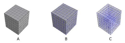
Figure 7.1: Hexahedral sampling method from B-Spline surfaces of degree 2. (A) 6 compatible B-Spline surfaces that bound a volume. Black lines delimit surfaces elements. (B) 6 quadrilateral meshes evaluated at physical positions of parametric values contained in vectors  $\mathcal{U}_q$  and  $\mathcal{V}_q$  of Equation (7.1) (quadrilateral meshes and points are depicted in blue). (C) Blue hexahedral patch computed using Coon's interpolation.
