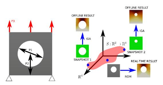
Figure 7.7: Reduced order model building and evaluation for a plate with one hole. Snapshots are calculated using isogeometric analysis. P1 and P2 are geometrical parameters defining respectively the diameter and the position of the hole along his height. P3 is a loading parameter. Response surfaces S are embedded in 4-dimensional space. There are as many surfaces as there are modes in the reduced basis.
