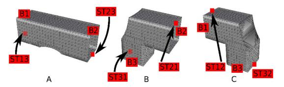
**Figure 3.6:** Boundary seed points computation. Temporary patches  $P_{T3}$ ,  $P_{T1}$  and  $P_{T2}$  respectively in (A), (B) and (C). Using an approach close to circular conformal mapping of [Zeng et al. 2009a], temporary seed points  $s_{Tk}$  are determined into each respective patch  $P_{Tk}$ .
