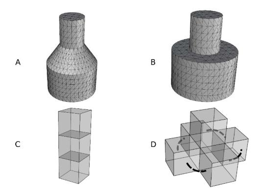
**Figure 6.7:** Volumetric layouts straightforward examples. (A) Triangulated mesh with sharp features. (B) Triangulated mesh with particularly marked sharp features. (C) Proposed volumetric layout for (A). (D) Proposed volumetric layout for (B).
