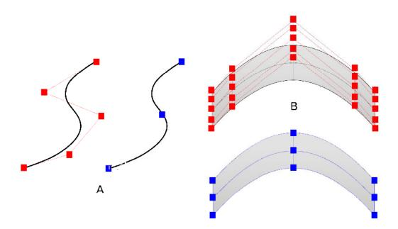
Figure 1.6: Cubic B-spline curve and surface. (A) A B-Spline curve with knot vector  $\Xi = \{0, 0, 0, 0, 1, 2, 2, 2, 2\}$ . (B) A B-Spline surface with knot vector  $\Xi = \{0, 0, 0, 0, 1, 2, 2, 2, 2\}$  and  $\mathcal{H} = \{0, 0, 0, 0, 1, 2, 2, 2, 2\}$ . Control points are depicted in red, whereas physical knot locations are in blue.
