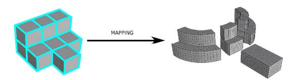
Figure 7.2: Volumetric isogeometric parameterization of the half-seal part for remeshing purposes. It is a genus-0 geometry with sharp features. Euler characteristic is  $\chi = -1$  for the mesh with 3 specially located boundaries. During the remeshing step, the parameterization is still the same whereas the geometry is changing under loading.
