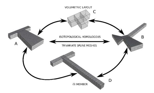
**Figure 6.9:** Isotopological isogeometric meshes constraints for reduced order modeling. (A) Isogeometric mesh with a geometry A. (B) Isogeometric mesh with a geometry B. (C) Associated volumetric layout of reference. (D)  $\alpha$ -member chosen to represent the whole population.
