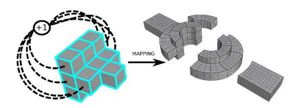
Figure 7.12: Volumetric isogeometric parameterization of the seal part. It is a genus-1 geometry with sharp features. Euler characteristic is  $\chi = 0$  for the associated closed mesh  $M_c$ . We apply the same parameterization among all members of the population to obtain isotopological comparable isogeometric meshes.
