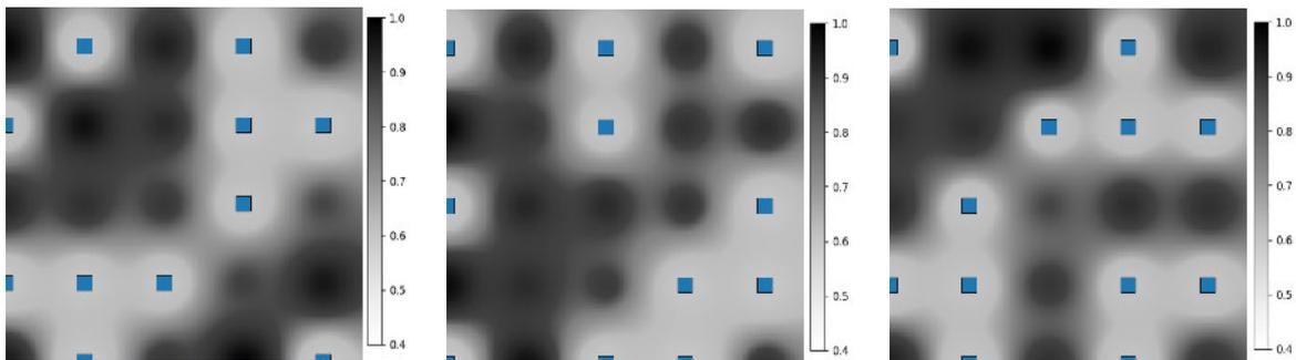
Figure 6.7: Proof-of-concept of the scheduling model: optimal WSN activity scheduling and the corresponding estimation errors' variance ( $\mu g^2/m^6$ ) while considering coverage requirements equal to  $1\mu g^2/m^6$ . Active sensors are depicted in blue squares.
