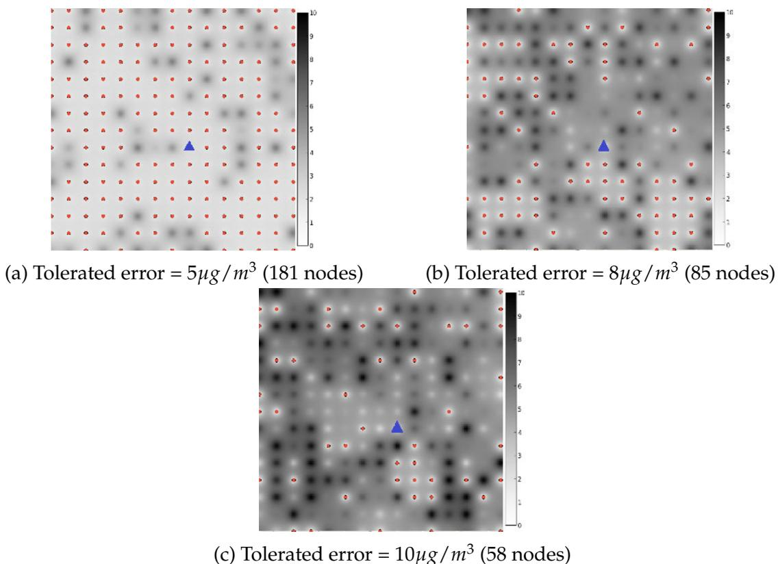
Figure 4.2: Proof-of-concept: Optimal WSN topology and the corresponding estimation errors ( $\mu\text{g}/\text{m}^3$ ) while considering different values of the maximum tolerated error. Sensors (respectively sinks) are depicted in red circles (blue triangles).
