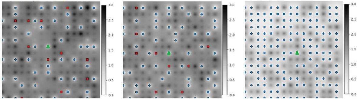
Figure 6.2: Proof-of-concept of the deployment model: optimal WSN topology and the corresponding estimation errors' variance ( $\mu g^2/m^6$ ) while considering different values of the deployment budget (from left to right: respectively 68, 75 and 155 monetary units). Sensors (respectively relay nodes and sinks) are depicted in blue circles (respectively red squares and green triangles). Note that the scale in these 3 figures is different than the scale of Fig. 6.1c.
