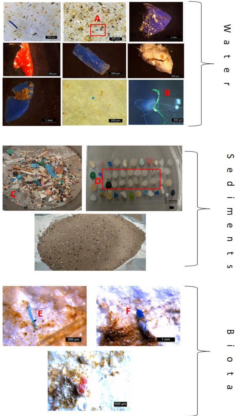
Fig. 3. Microplastics of different shapes and colors collected along the Lebanese coast in three different matrices: e.g. A) blue microbead and B) green fiber found in the collected surface water, C) Macro and microplastics collected on the 2 mm sieve and D) white and black pellets collected in Tripoli sediments sample, E) blue fiber and F) blue fragment observed on biota filter.
