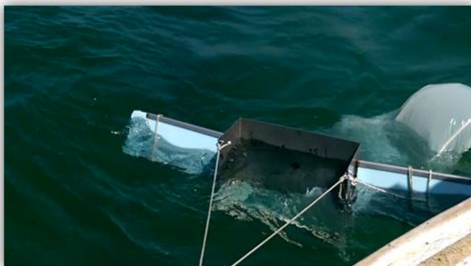
Figure 17: Manta trawl used in collecting the water samples off the Lebanese coast.
