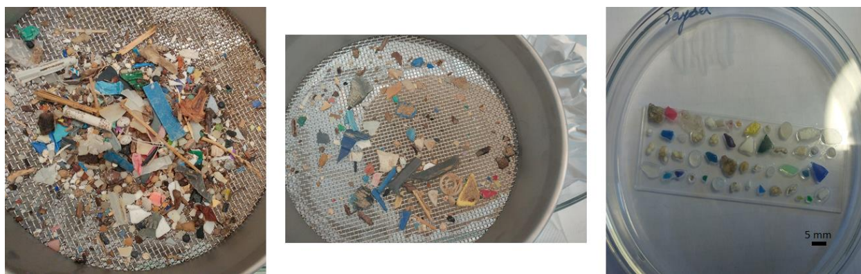
Figure 29: Sieved sediment on a 2 mm mesh size and visually sorted on a microscopic slide for Raman analysis.
