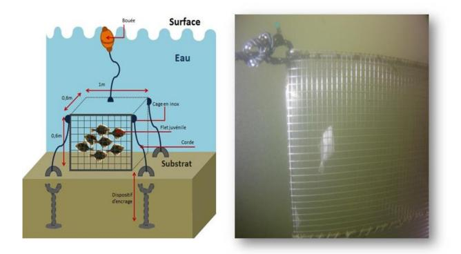
*Figure 24:* Caging model and real photos of cages constructed for Platichthys flesus deployed in three different estuaries along the Eastern English Channel
