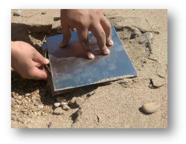
*Figure 19:* Steel ring with two stainless-steel plates used in collecting sediments along the Lebanese coast.
