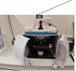
*Figure 36: Micro-Raman Xplora Plus (Horiba Scientific, France) used for microplastics identifying throughout this thesis. The open door (on the left) is closed (on the right) during samples analyses (limiting airborne contamination to filters).*
