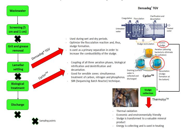
*Figure 15:* Wastewater treatment steps inside Edelweiss WWTP with the different treatment phases and characteristics the water undergoes. Also, the three sampling points are indicated in the diagram (adapted from Edelweiss, 2016).
