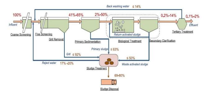
*Figure 41:*Estimated microplastics particle flow in wastewater treatment plant with primary, secondary and tertiary treatment process (source: Sun et al., 2019)
