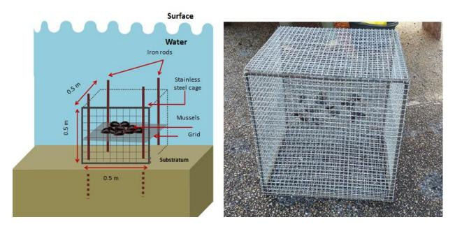
*Figure 26:* Caging model and real photos of cages constructed for Mytilus edulis deployed in Le Havre harbor and Sainte-Adresse.
