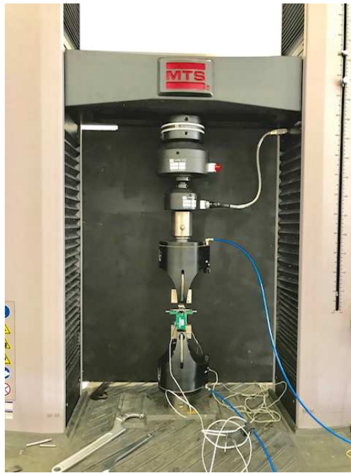
Figure 3.62: Experimental setup in FEMTO-ST (Besançon) for the quasi-static measurement of the Young's modulus
