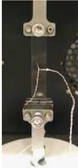
Figure 3.88: Setup for the measurement of \tau_{th}
