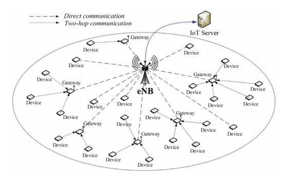
Figure. I.2: LTE-M network architecture [66]
