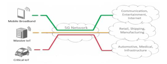
Figure. I.7: Network Slicing architecture
