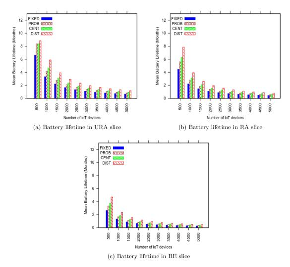
Figure. IV.6: Mean Battery lifetime in every slice with various slicing strategies
