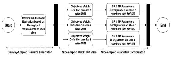
Figure. III.3: The proposed slicing and TOPG optimization algorithm
