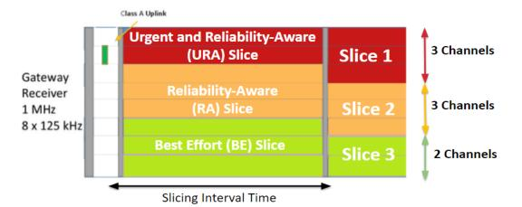
Figure. II.1: Channels slicing example over a LoRa GW
