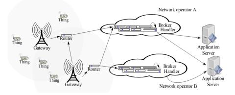
Figure. I.5: LoRaWAN architecture [10]
