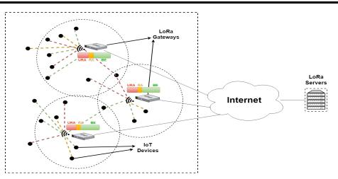
Figure. II.2: IoT slicing architecture in LoRa networks
