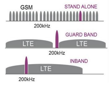
Figure. I.1: Operation modes in NB-IoT [59]
