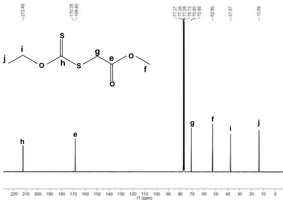
Figure 2.5: ^{13}\text{C} NMR spectrum of RAFT agent methyl [(ethoxycarbonothioyl)]sulfanyl acetate ( \text{CDCl}_3 , r. t.).
