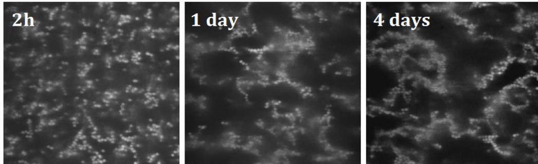
Figure 2.13 – Structural evolution during aging of a tenuous depletion gel. Figure taken from [126].
