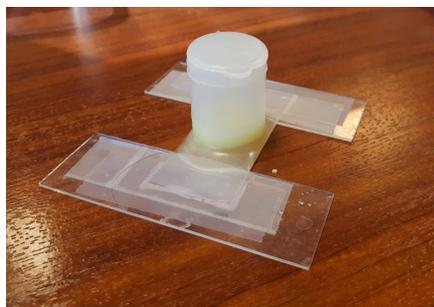
Figure 3.20 – A typical sample cell used for imaging. The suspension is inserted into a sealed plastic vial laying on a microscope coverslip.
