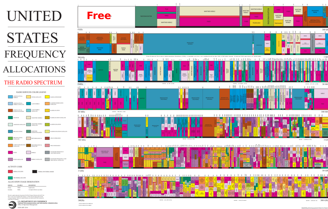
Figure 1.1 – A chart representing the allocation of radio spectrum in the United States of North America in 2016. © United States of North America, Department of Commerce, published online at www.ntia.doc.gov/files/ntia/publications/january_2016_spectrum_wall_chart.pdf .
