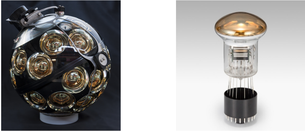
Figure 3.2: Photographs of a KM3NeT DOM (left) and Hamamatsu R12199-02 photomultiplier tube (right). In the DOM, the visible part of the individual PMTs comprise the photocathode areas, circled by the silver-coloured reflector rings.
