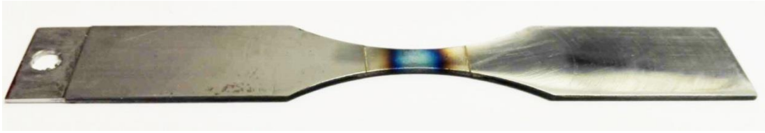
Figure 3.13 Photo of \alpha -iron specimen after successive self-heating tests displayed in Figure 3.11a.
