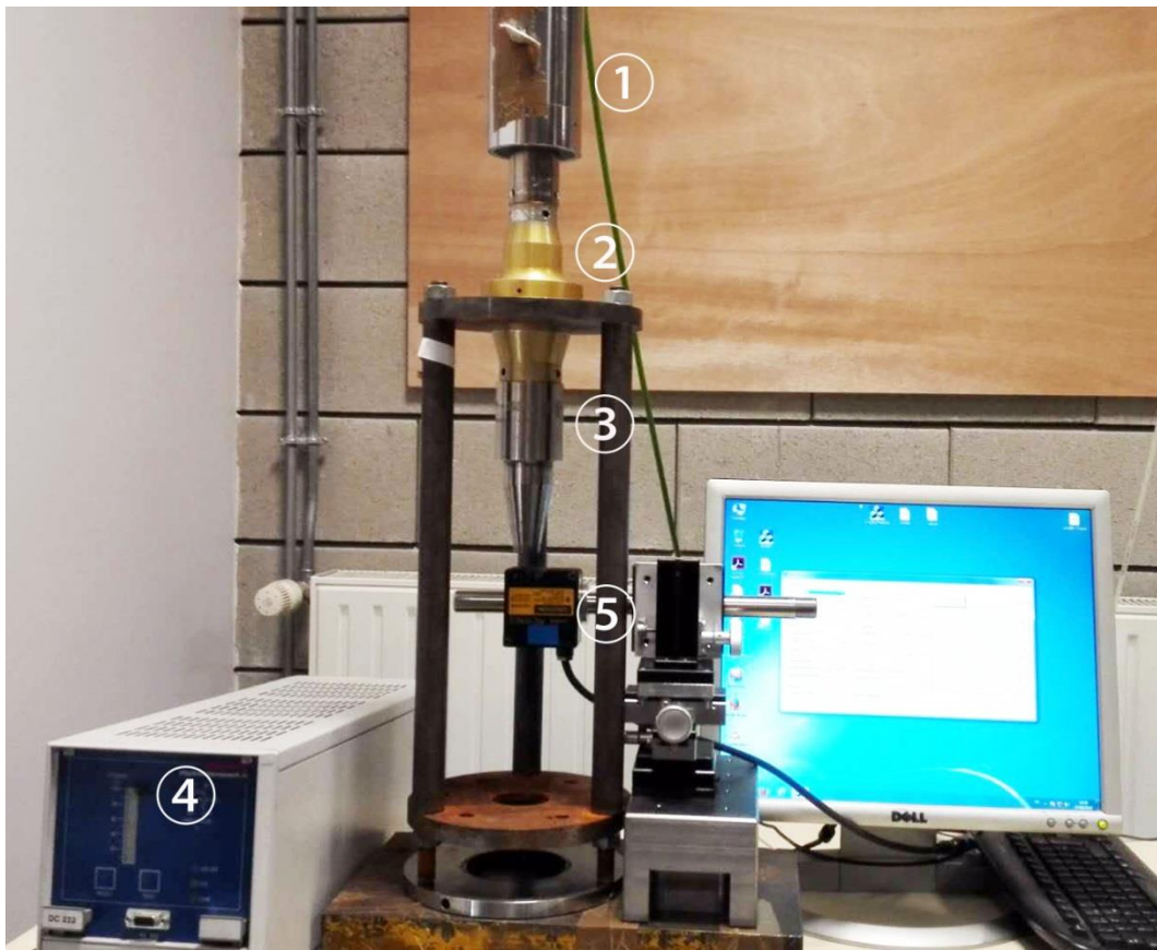
Figure 2.1 Components of fatigue system: ①converter, ②amplifier, ③horn, ④generator, ⑤ laser sensor.
