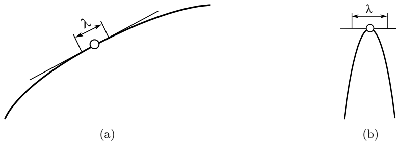
Fig. 1.7 The tangent plane approximation is a consistent approximation in the case of a small slope (a), but is rather inconsistent in the case of an abrupt slope (b). Schema reproduced from [11].
