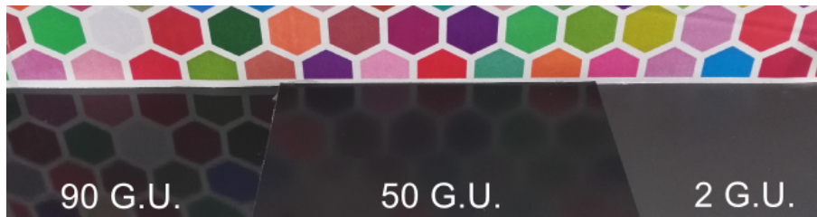
Fig. 4.8 Photograph of three samples of the 3C Conseil scale, with Gloss Unit of 90, 50 and 2, observed in a light booth (Spectralight QC X-Rite), under D65 illumination.
