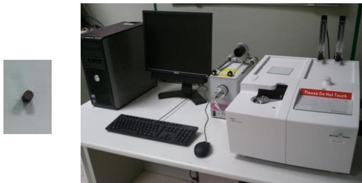
Figure 57. Thermal diffusivity characterization sample (left) and device for its calculation (right)
