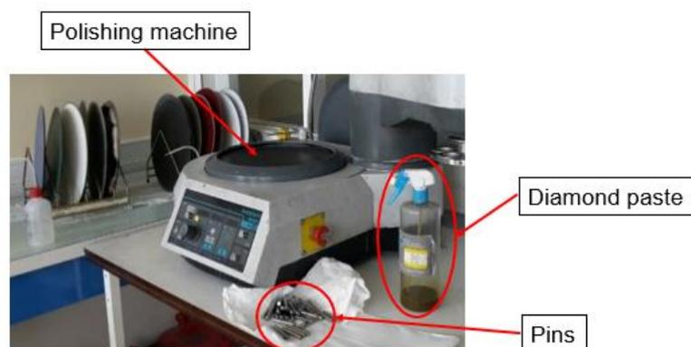
Figure 87. Polishing device and paste used to clean the pins.
