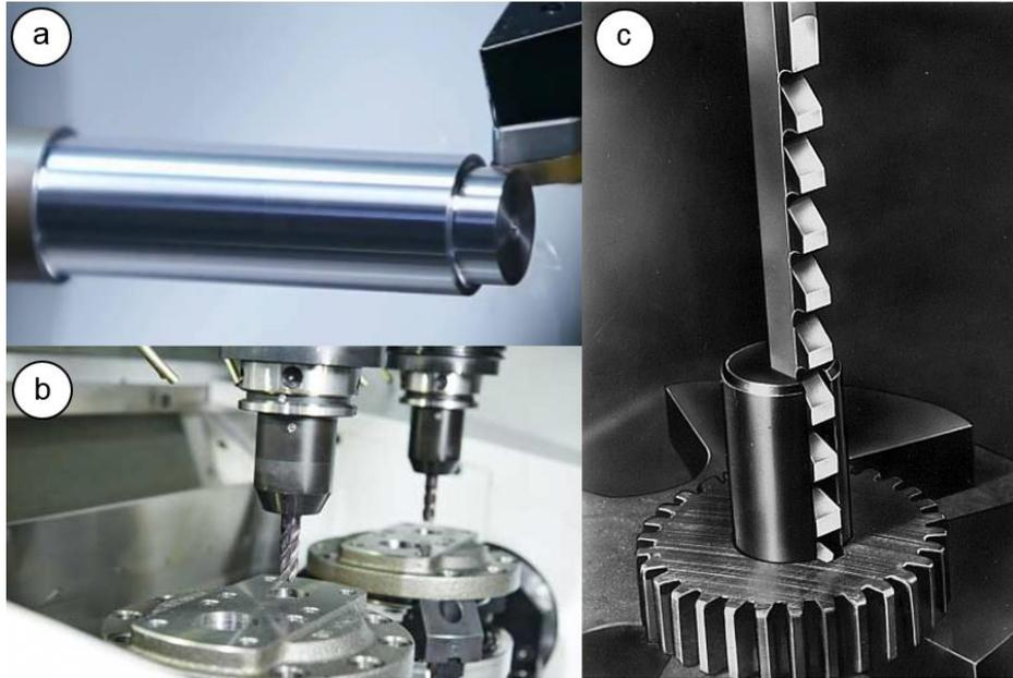
Figure 2. Turning, drilling and broaching processes.
