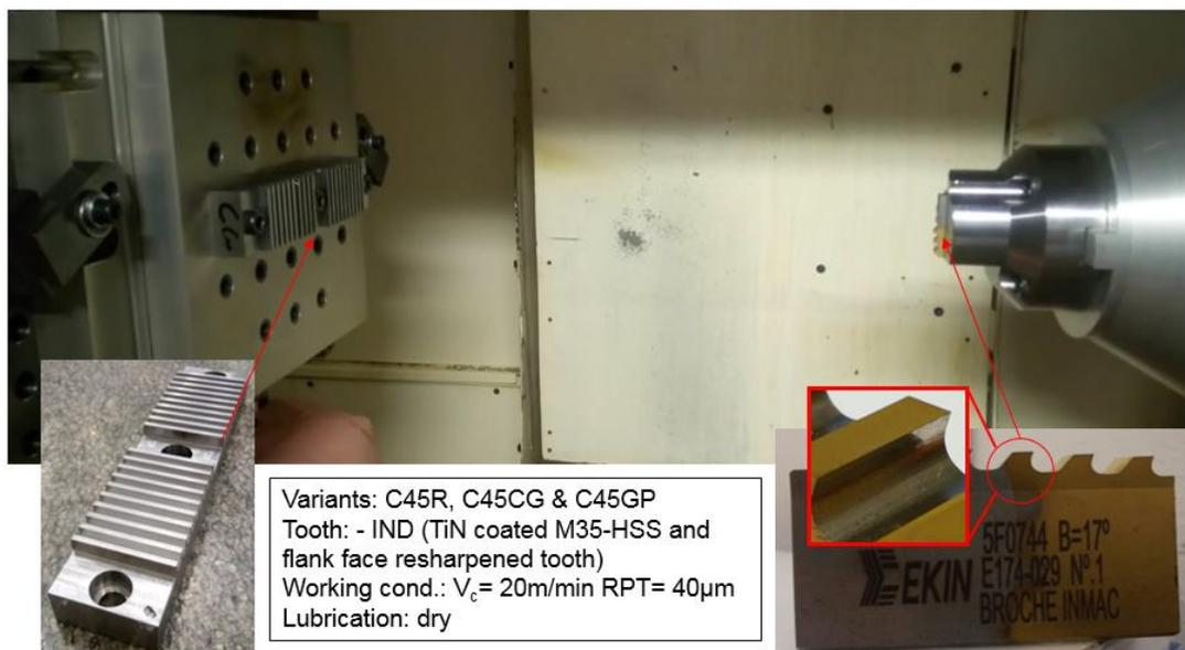
Figure 153. Broaching setup vertically mounted showing the wear tests sample and sued tooth.
