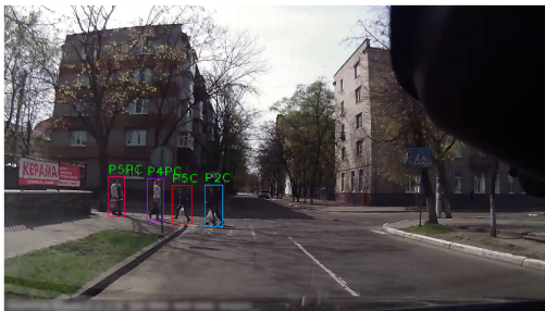
(g) Results of pedestrian detection using PPC, PC, PAC, PA classes and pedestrian ids.
