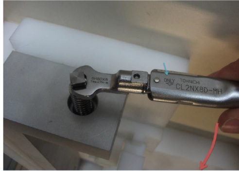
Figure 3.3.10: Tightening the screw with the torque wrench.
