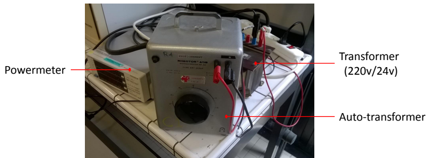
Figure 3.3.5: Voltage magnetization set-up.
