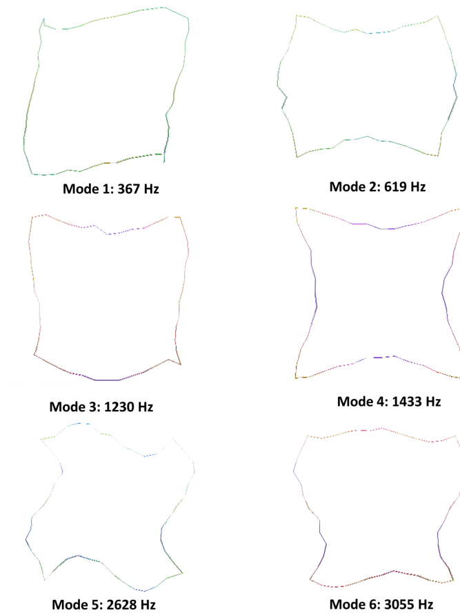
Figure 4.4.8: In-plane modes shapes (measured).
