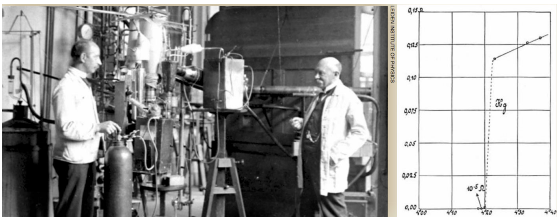
FIGURE 5.1: The liquid helium experiment of Heike Kamerlingh Onnes (on the right) and his chief technician Gerrit Flim. The historic superconducting plot of resistance versus temperature of the mercury at low temperature.
