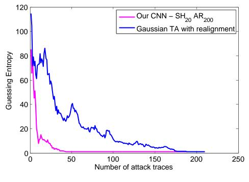
FIGURE 6.11: Comparison between a Gaussian template attack with realignment, and our CNN strategy, over the modern smart card with jitter.
