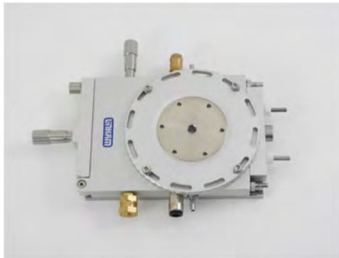
FIGURE 2.29 – Platine chauffante Linkam THMS 600
