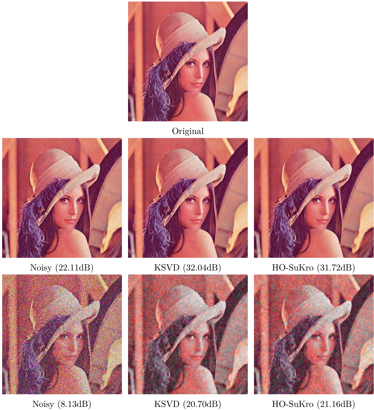
Figure 6.11 – Examples of denoised images for input PSNR of 22.11dB and 8.13dB respectively at second and third rows.
