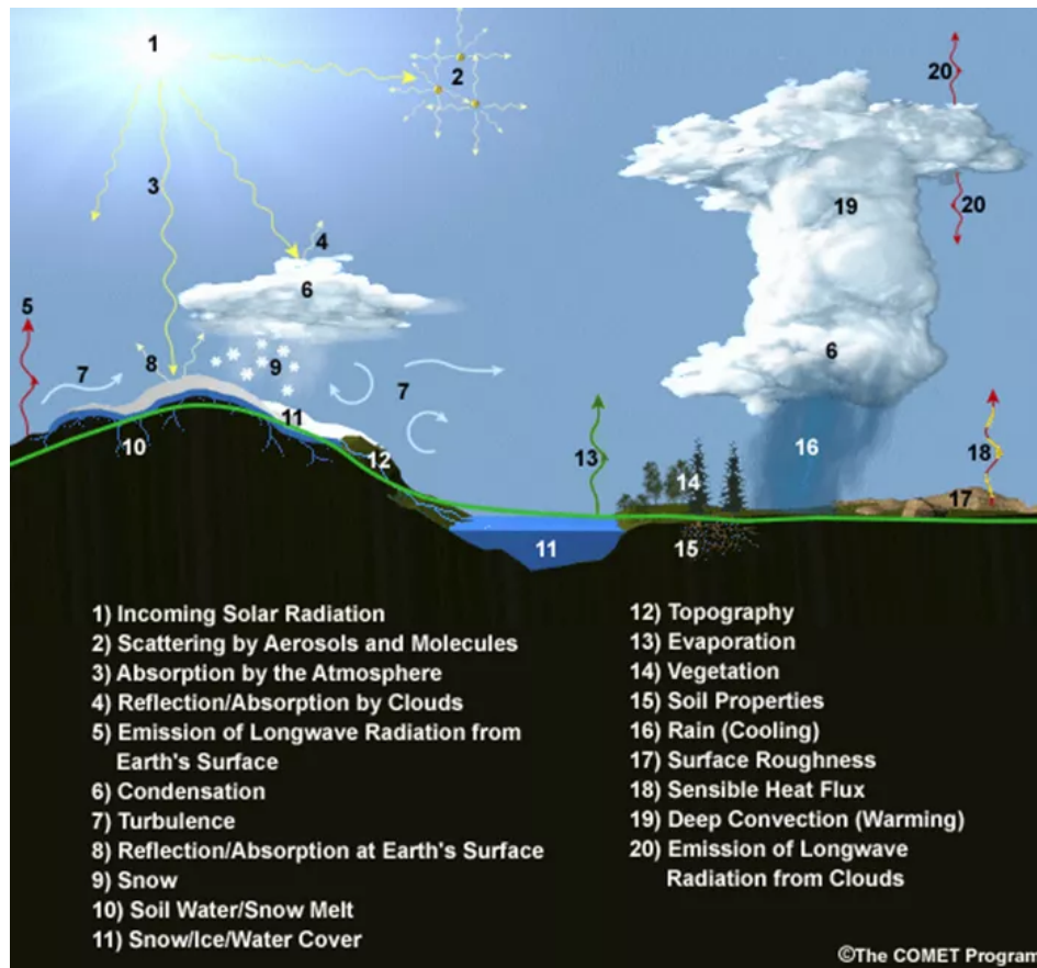
Figure 1.8 – Illustration of some of the atmospheric processes that are typically parameterised in NWP models. Image courtesy of MetEd, The COMET Program, UCAR.
