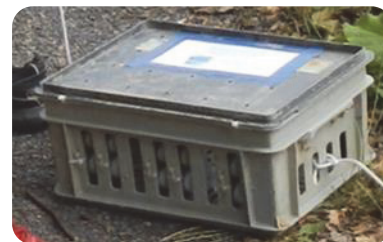
Figure S1: Exposure systems for DGT deployed on the Gier River (a) and on the Deûle River (b)
