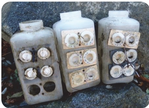
Figure S1: Exposure systems for DGT deployed on the Gier River (a) and on the Deûle River (b)
