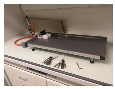
FIGURE 5.1: Tape casting setup.
