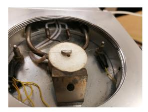
FIGURE 3.1: Picture of the impedance measurement device (Linkam).
