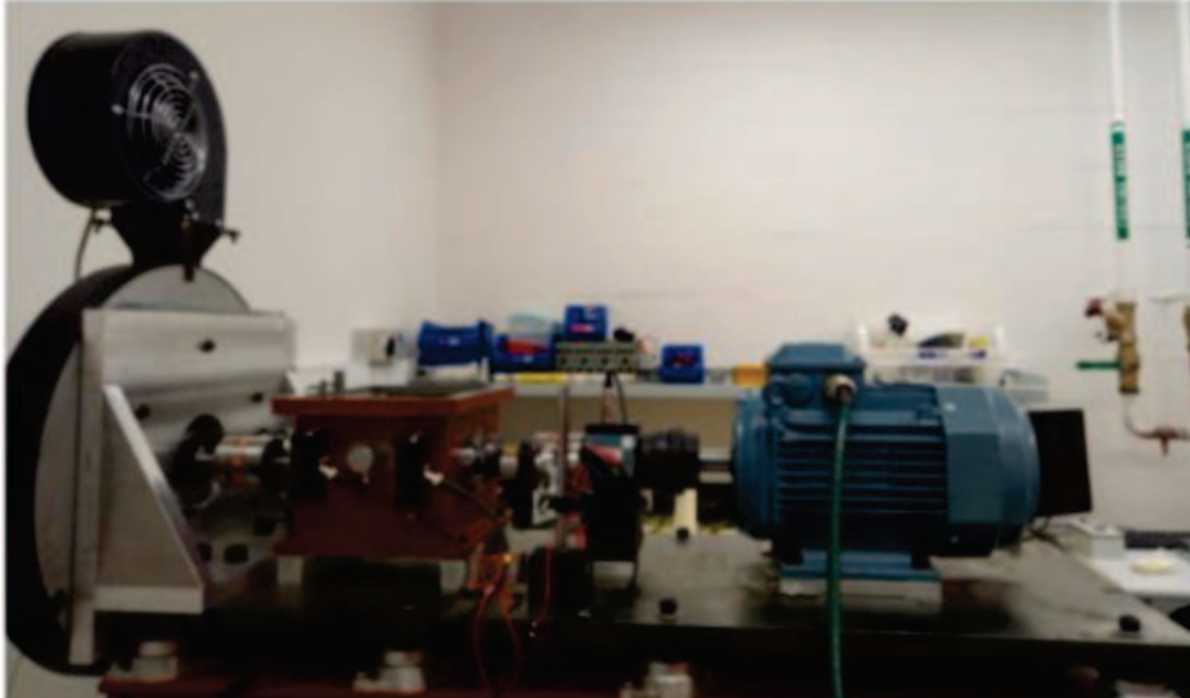
Figure 8.1: The spur gear test rig at the University of New South Wales (UNSW).
