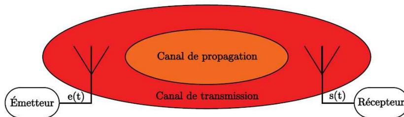
Figure 1-31: Canal de propagation et canal de transmission [130]
