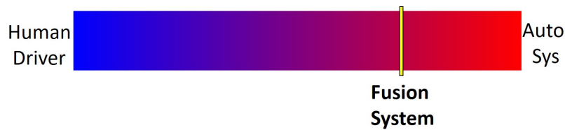
Figure 1.15 – An example of the division of control authority between human and autonomous driving system using fusion system
