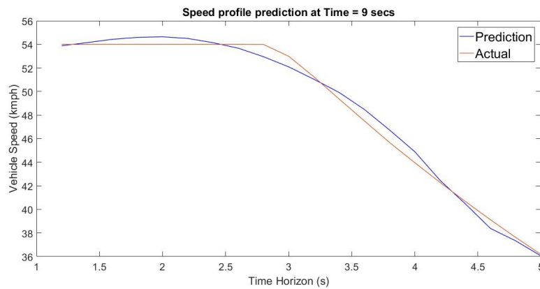
Figure 4.15 – Use Case 1: Vehicle Speed Profile prediction at time = 9 secs
