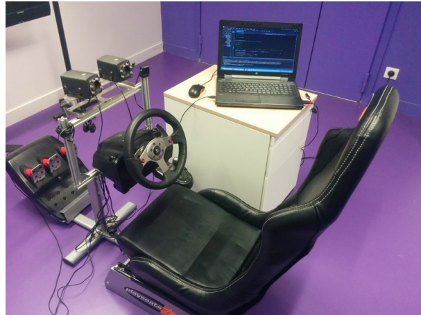
Figure 4.9 – Driving Simulator Platform at Heudiasyc Laboratory
