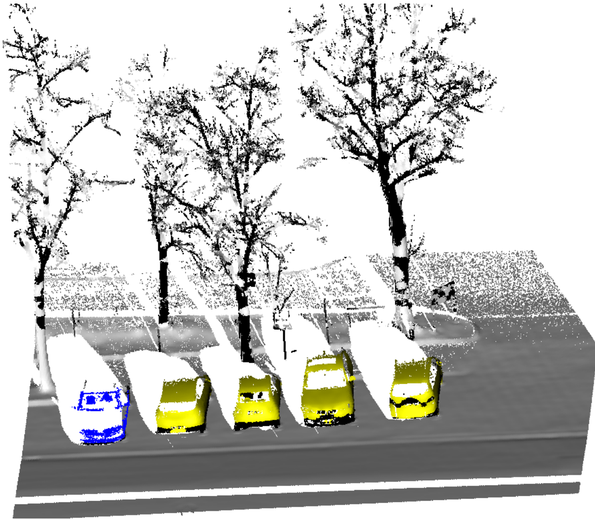
Figure 11.7: Example of a point cloud containing cars that have been detected (yellow) and not detected (blue) before the learning process.
