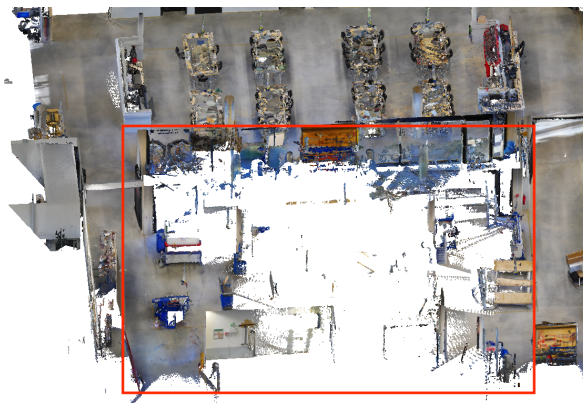
Figure 4.6: Point cloud of a room with a missing part due to the influences of external factors.
