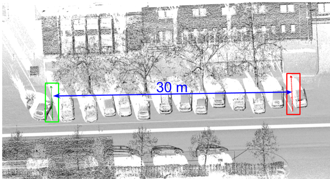
Figure 10.6: Illustration of the inference of the position of a street light (in red) thanks to the detection of another street light (in green) and its topological link (in blue).
