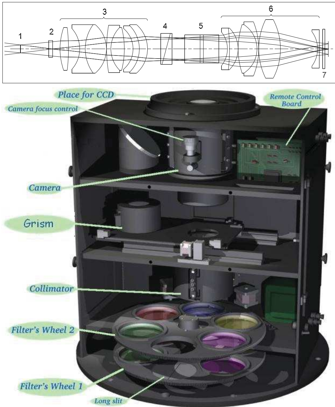
Figure 6.6: Upper panel: the optical scheme of the polarimetric mode of the focal reducer SCORPIO: 1–slit; 2–the phase plate; 3–the collimator, 4–the Wollaston prism; 5–the grism; 6–the spectrograph camera; 7–the entrance window of the CCD (charged coupled device) cryostat. Credits: Afanasiev & Amirkhanyan (2012). Bottom: a real picture of SCORPIO with all its optical elements marked in the figure. Credits: SAO RAS gallery https://www.sao.ru/hq/lsvfo/devices/scorpio/scorpio.html .
