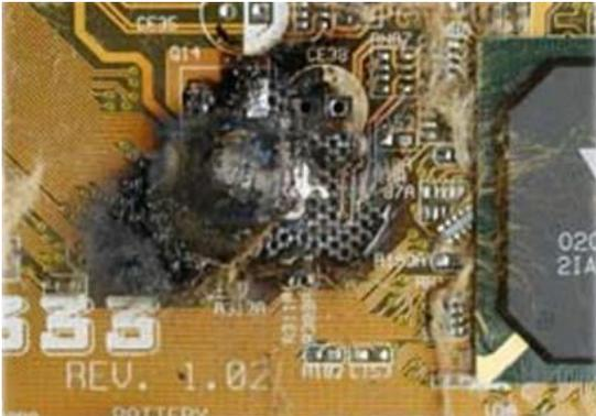
Fig. 12. Capacitor burned due to supraharmmonic emissions [62].
