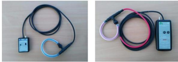
Fig. 21. LFR 06/6 and CWT015 used in channels 3 and 4.
