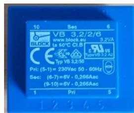
Fig. 42. VT used in channel 1.
