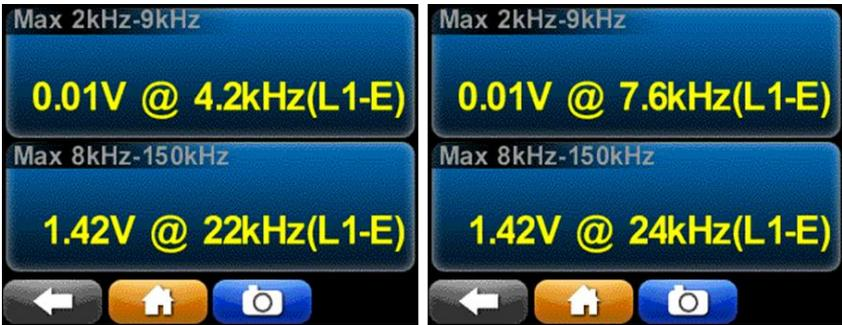
Fig. 14. PQube 3 output for voltage supraharmonic emission at 23 kHz.
