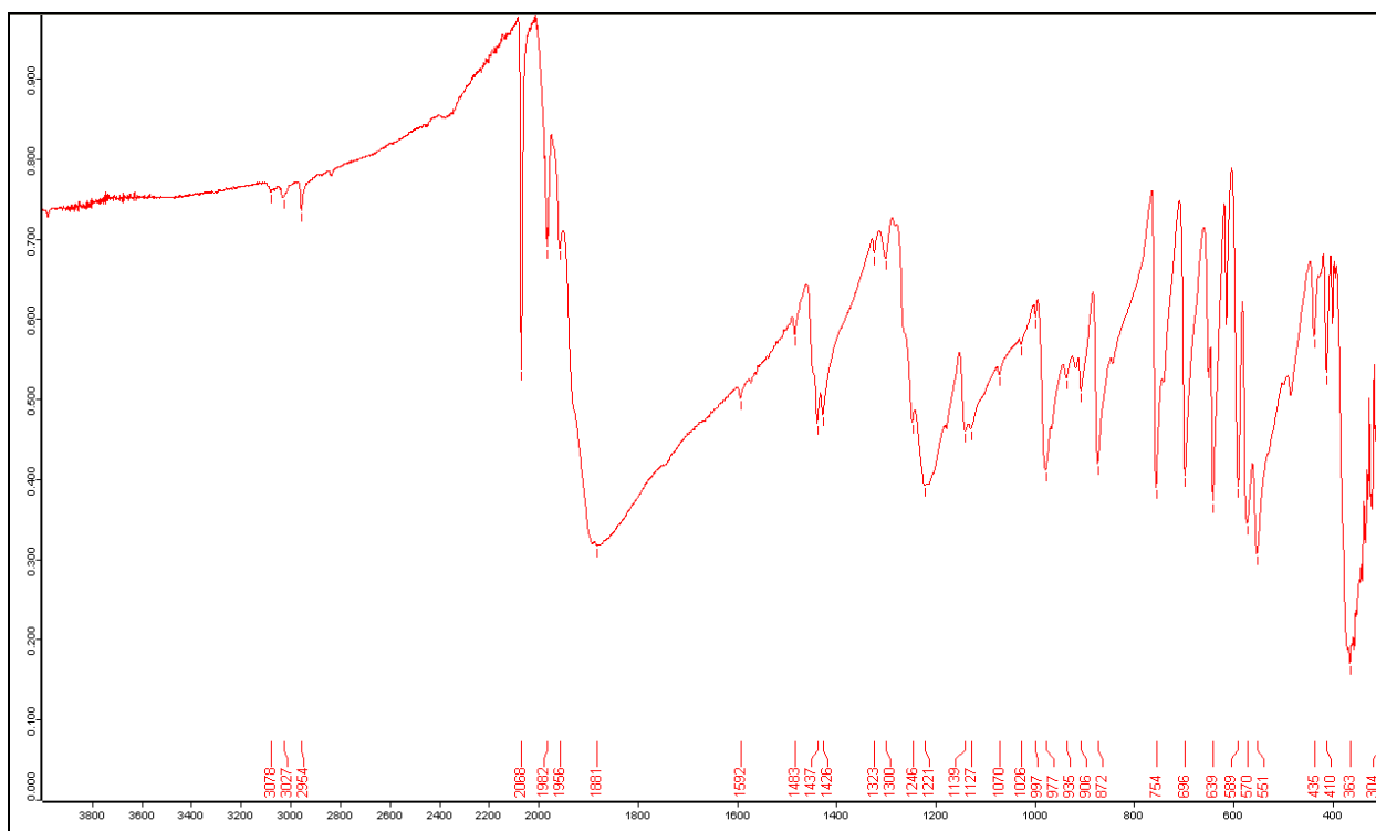
Figure SI 3.22 IR solid state (powder) spectrum of the Fischer carbene 3.2c .
