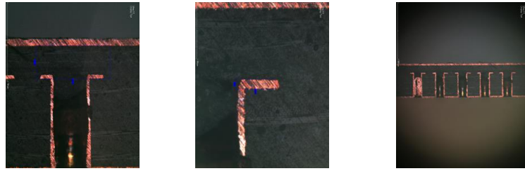
Figure 2-21: Cross-section view (Photograph) of internal metallized via holes
