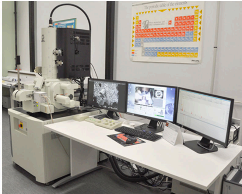
Figure 2.5. Zeiss SUPRA 55 scanning electron microscope.
