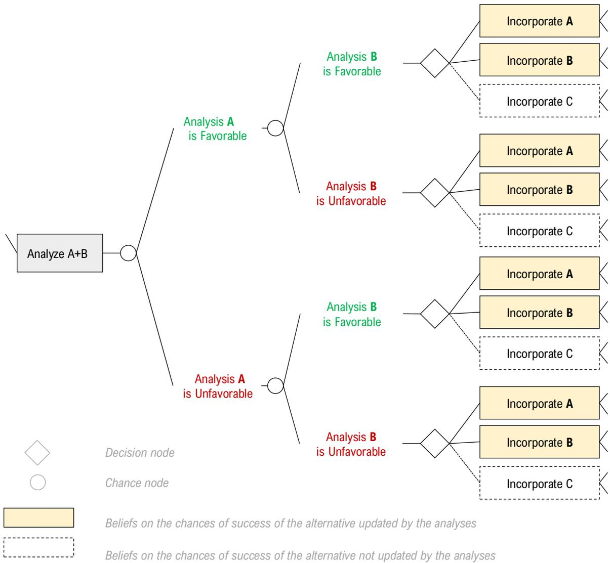
Figure 11 - Structure of "Analyze in parallel" alternative: example with Solutions A and B
